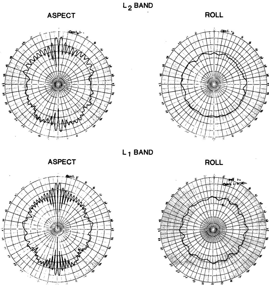
**FIGURE 4. MEASURED ANTENNA PATTERNS, L<sub>1</sub> AND L<sub>2</sub>**
