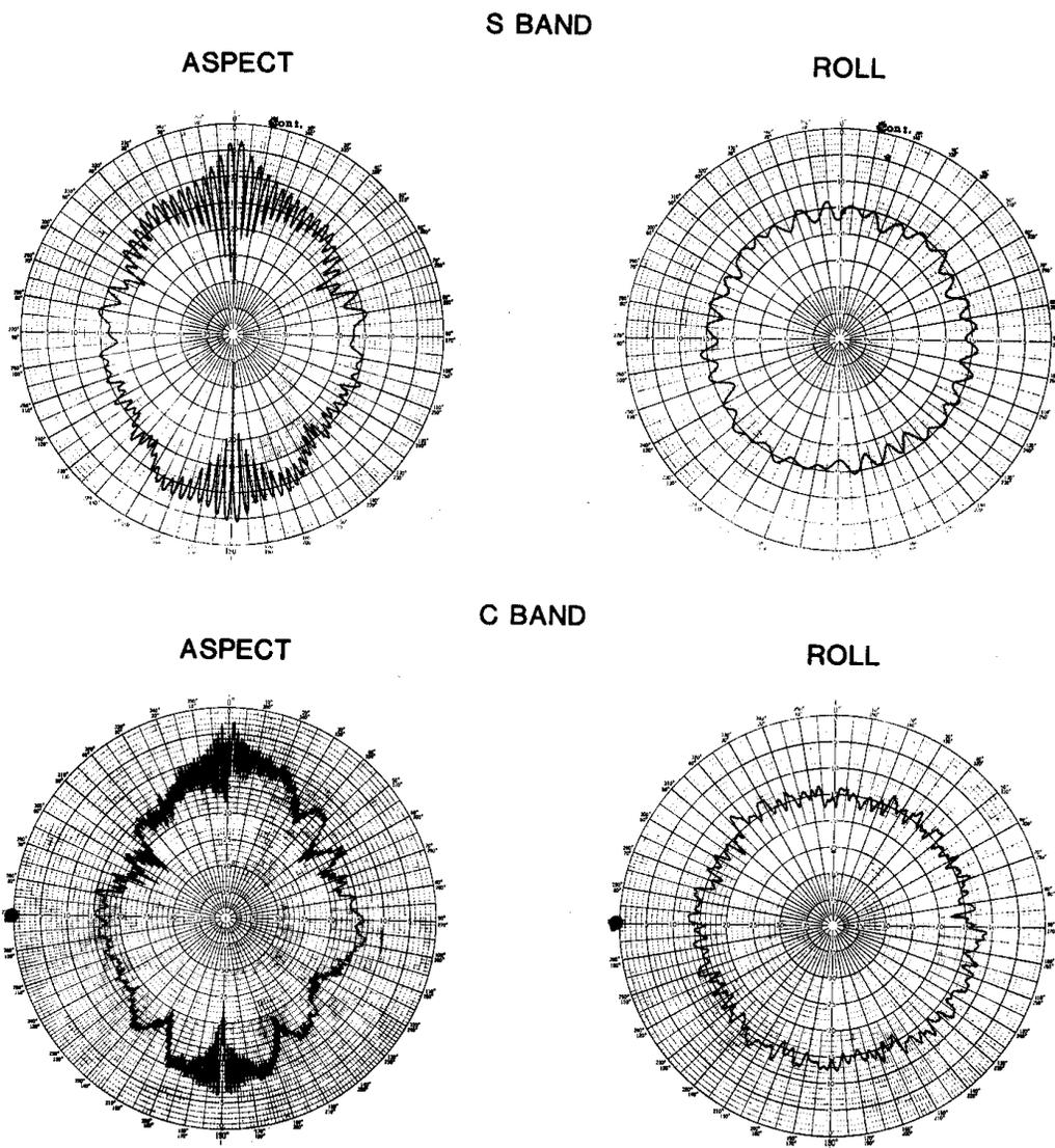
**FIGURE 5. MEASURED ANTENA PATTERNS, S AND C**
