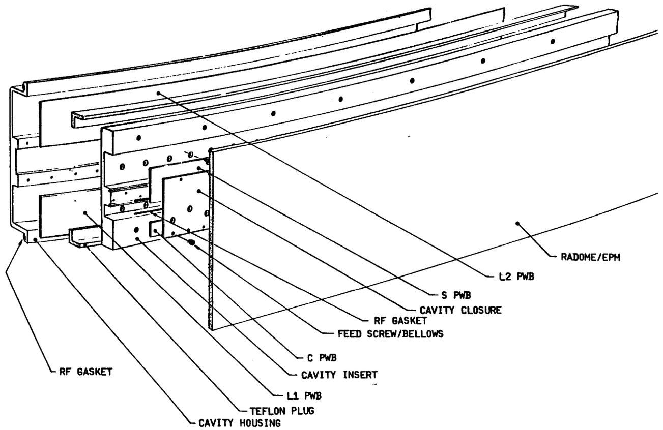
**FIGURE I ANTENNA SEGMENT CONFIGURATION**
