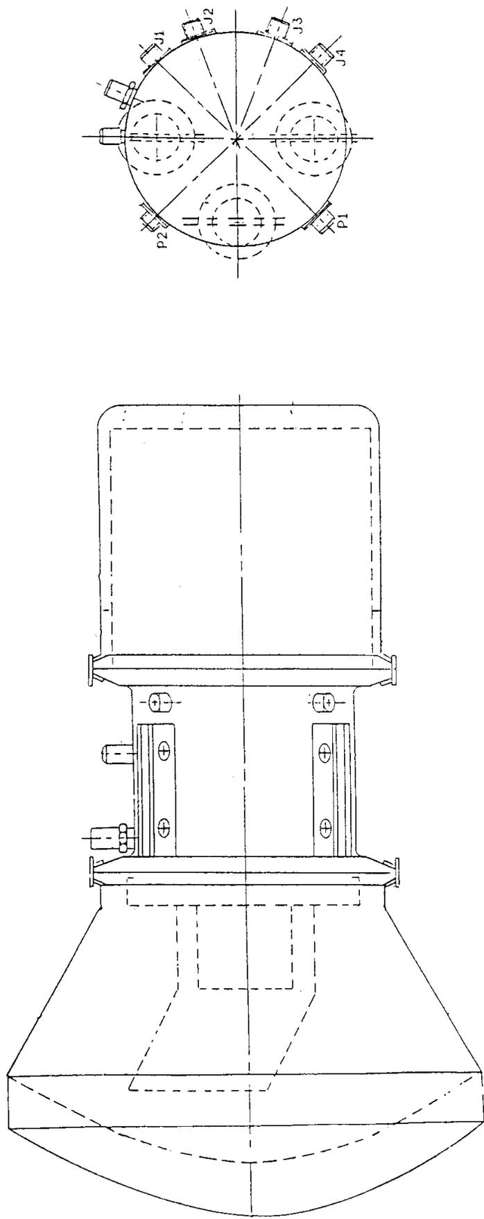
**FIGURE 3; RADSCAN FEED (MODIFIED RADOME)**
