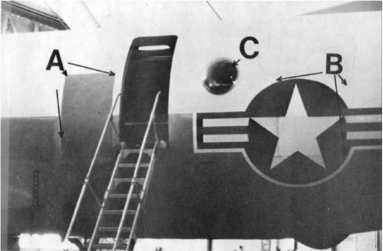
**Figure 2. Conformal Microstrip Mobile Receive Telemetry Antenna Mounted on P-3 Aircraft**
