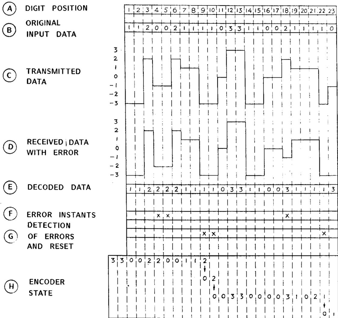
FIGURE 4 ERROR DETECTION FOR  $R = 4$
