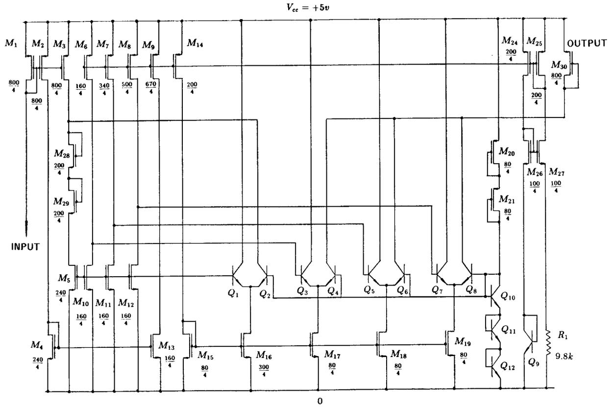
**FIGURE 1 BI - CMOS QUATERNARY MODULAR ADDER**
