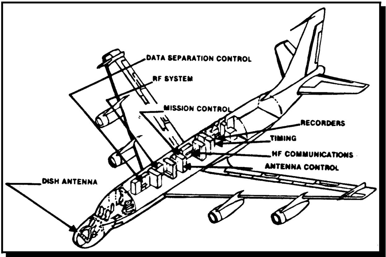
**FIGURE 1 - ARIA PMEE SUBSYSTEMS**
