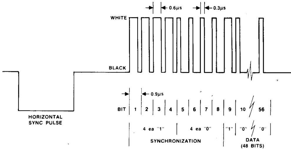
**FIGURE 1 TIMING FORMAT WAVEFORM**
