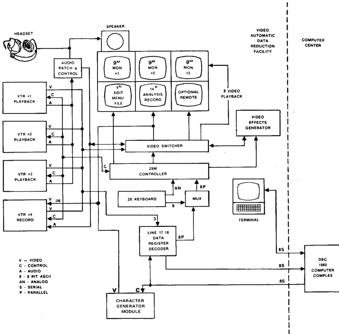
**FIGURE 6 SIMPLIFIED BLOCK DIAGRAM VIDIO EDITING FACILITY**
