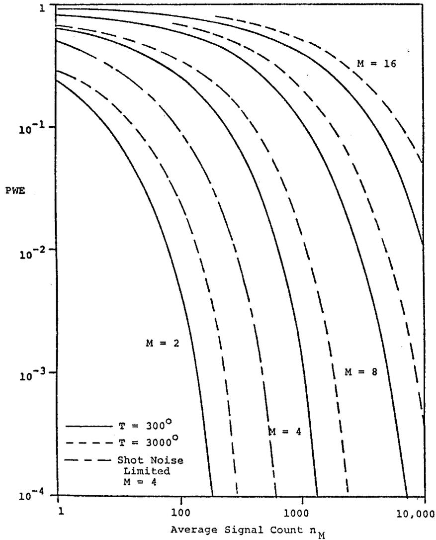
**Figure 3. M-ary PIM Performance (Additive Thermal Noise, Non-Linear Intensity Levels, Optimum Gain  $G$  Selected)  $k = .028$ ,  $R = 50$  ,  $B = 1000$  MHz.
