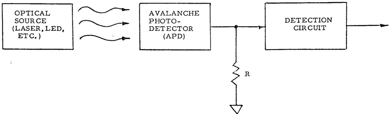
**FIGURE 2 -- AVALANCHE PHOTO-DETECTION MODEL (APD)**
