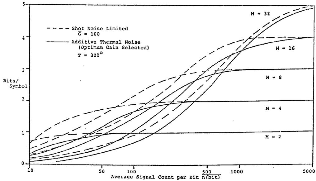
**Figure 4. M-ary PIM Mutual Information as a Function of Average Signal Count per Bit.  $k = .028$ ,  $R = 50$  ,  $B = 1000$  MHz.  $\bar{n}_b$  (back round noise = 1**
