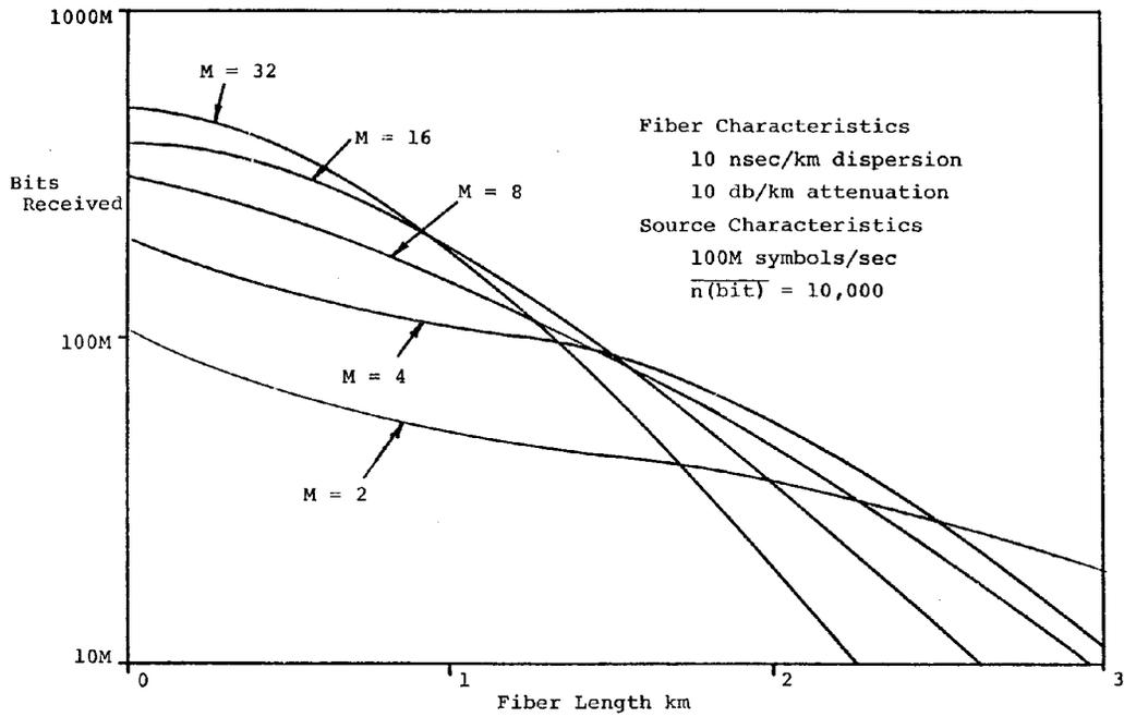
**Figure 6. M-ary PIM Fiber Link (Bits Received per Fiber Length, Additive Thermal Noise)  $\bar{n}_b = 1$ ,  $k = .028$ ,  $T = 300^\circ$ ,  $R = 50$ ,  $B = 100$  MHz, Non-Linear Intensity Spacing, Optimum Gain Selected.**
