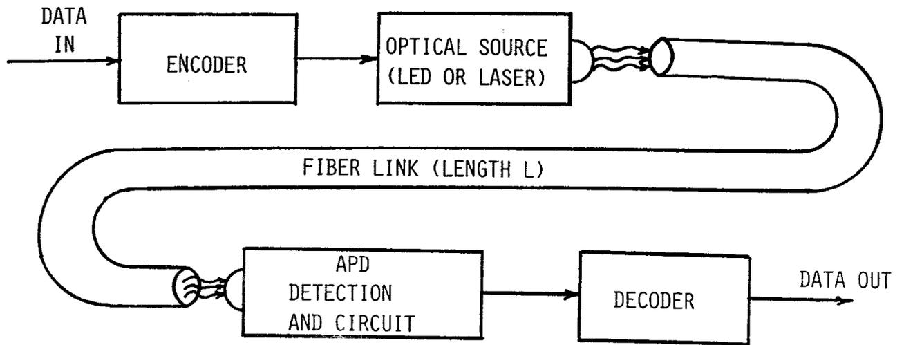
**FIGURE 1 -- ENCODED DIGITAL FIBER LINK WITH AVALANCHE PHOTO-DETECTION (APD)**
