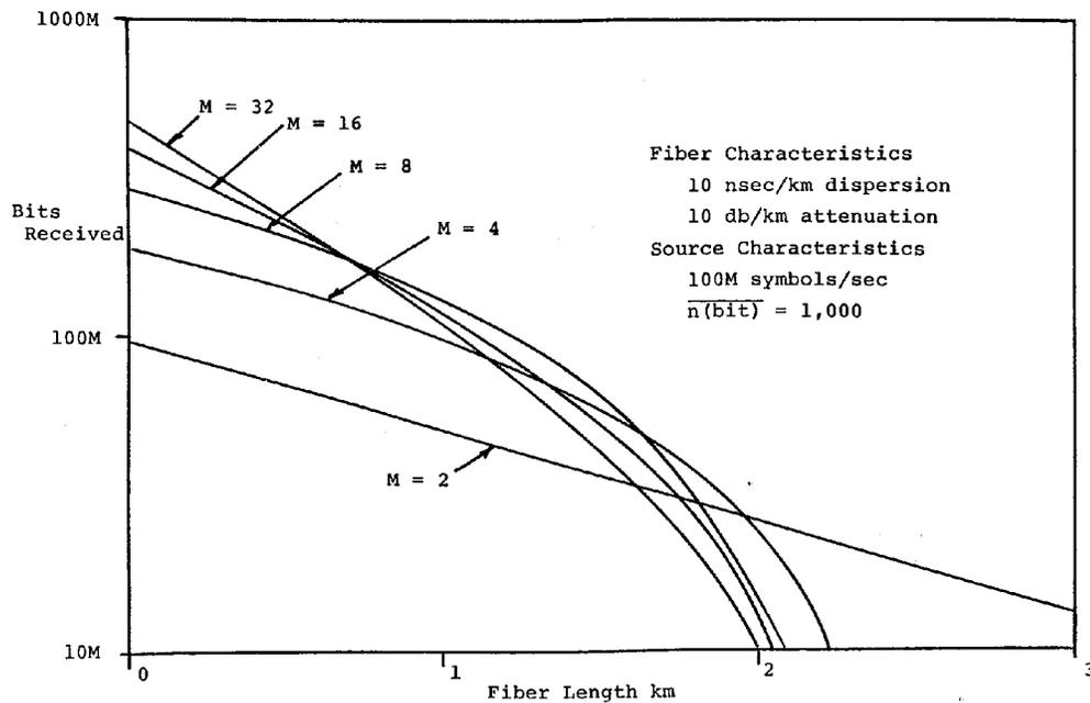
**Figure 5. M-ary PIN Fiber Link (Bits Received per Fiber Length, Shot Noise Limited)  $\bar{n}_b = 1$ ,  $k = .028$ , Non-Linear Spacing, Optimum Gain Selected.**
