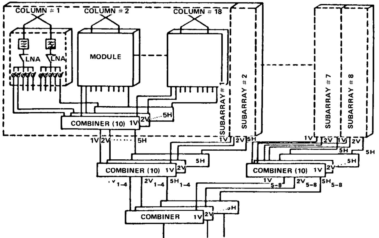
FIGURE 6. ARRAY ANTENNA RF NETWORK
