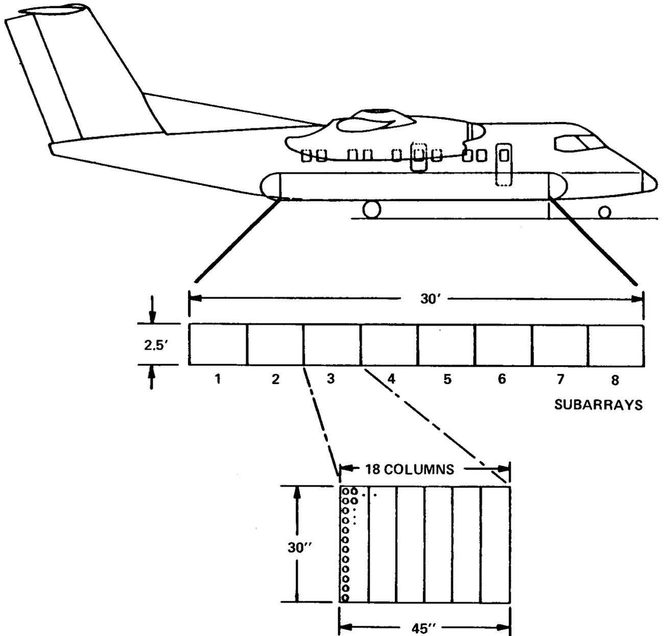
**FIGURE 5. MECHANICAL LAYOUT OF S-BAND TELEMETRY PHASED ARRAY ANTENNA**
