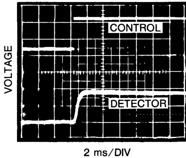
Figure 12. Measured MPLL
