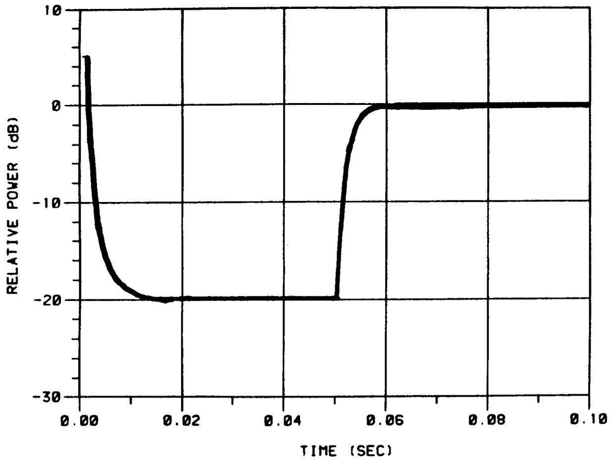
Figure 11. MPLL Step Response Simulation
