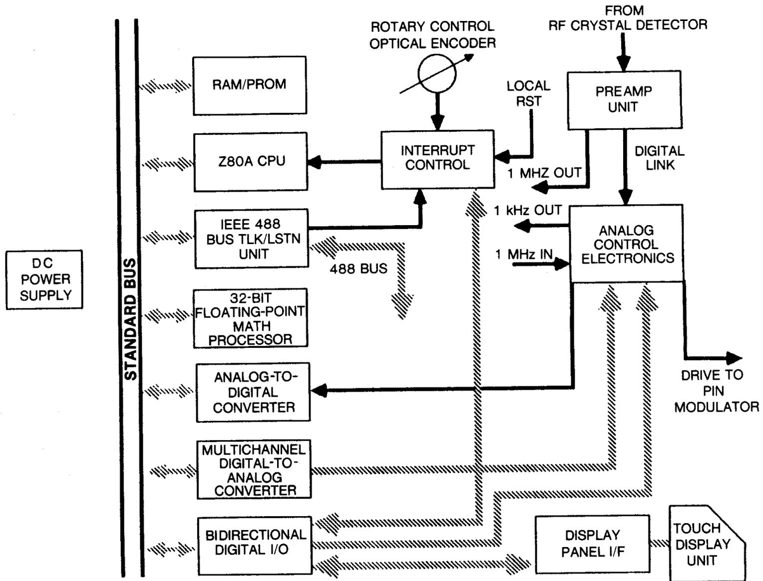
Figure 4. MPLL Block Diagram
