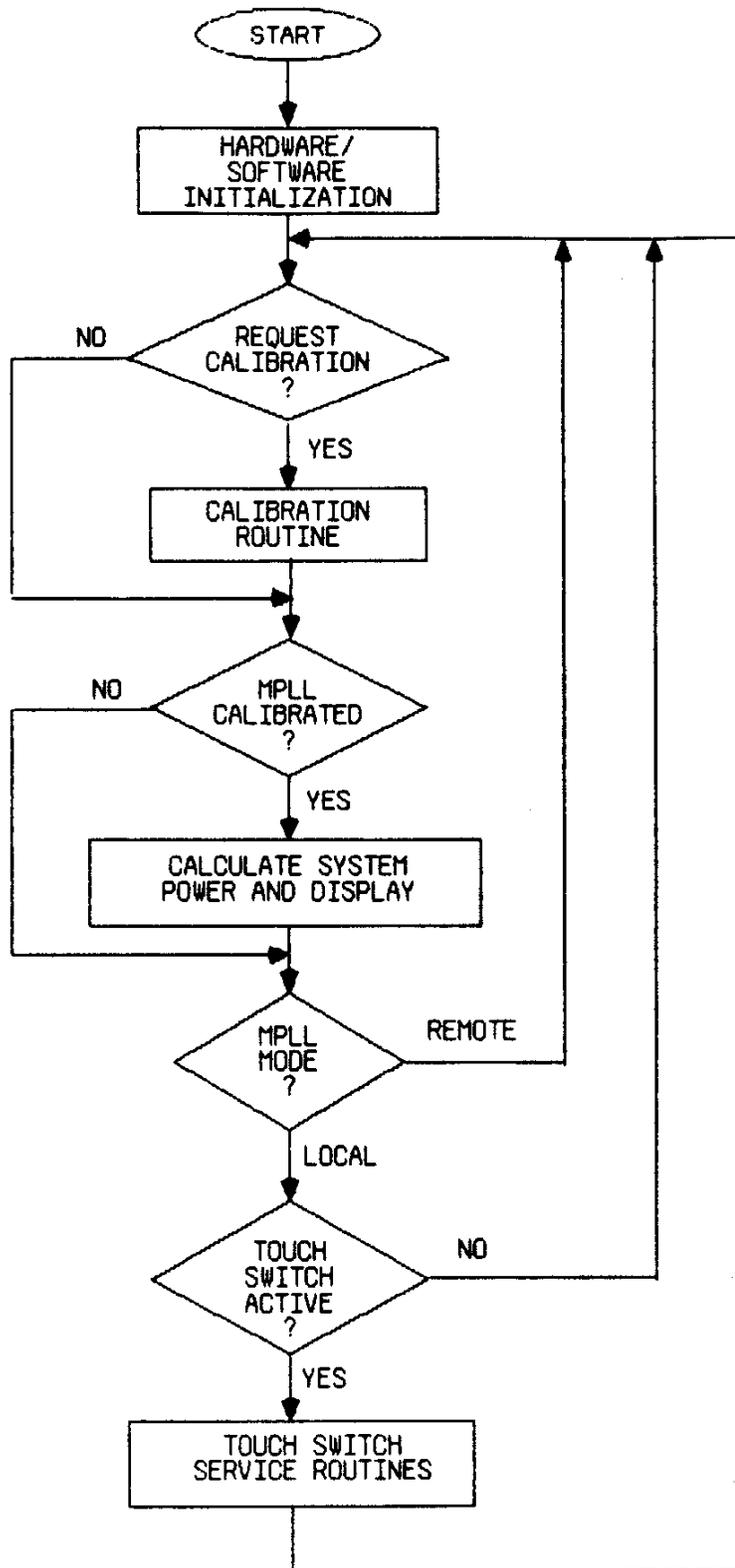
Figure 6. MPLL Software Flow
