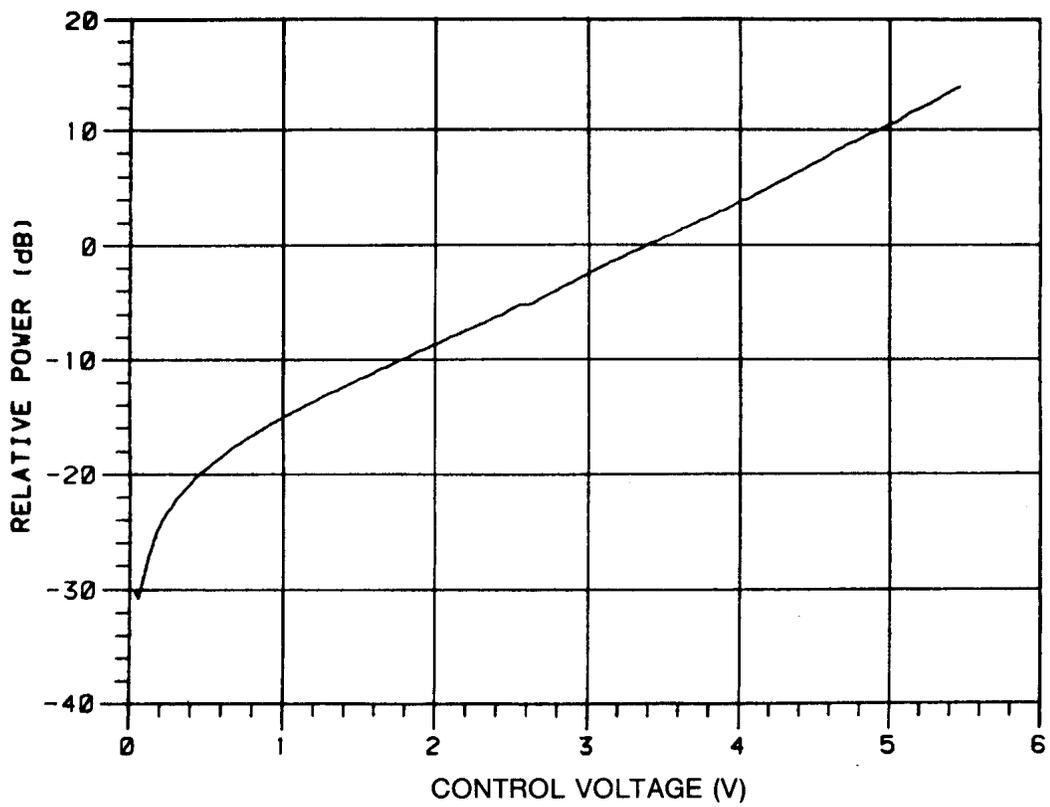
**Figure 13. MPLL Transfer Function Simulation**
