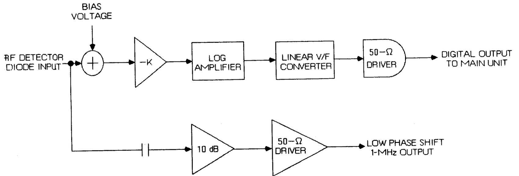
**Figure 3. Preamp Block Diagram**
