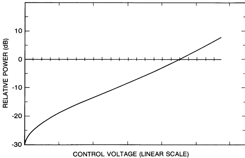
**Figure 14. Measured MPLL Transfer Function**
