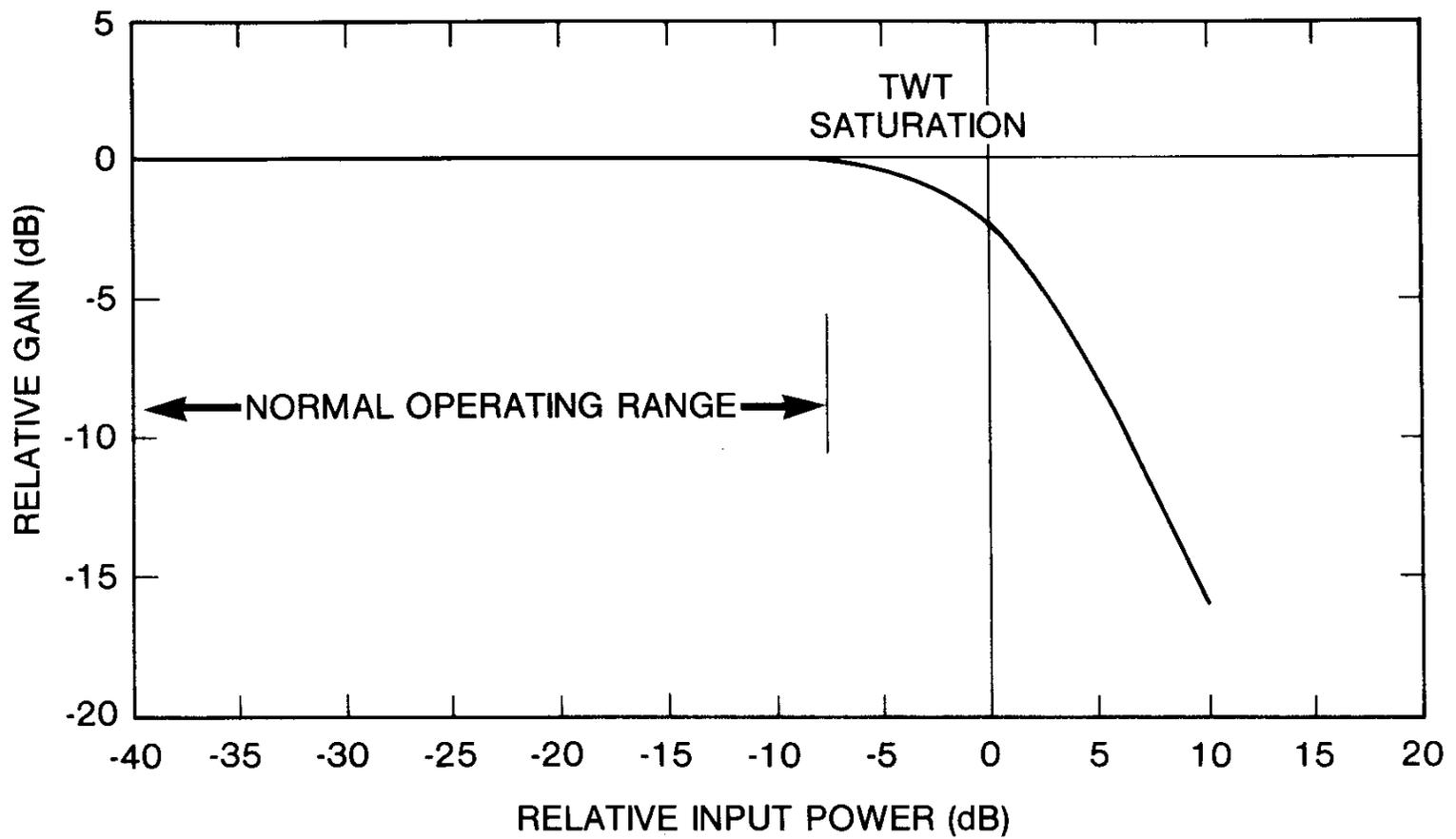
**Figure 10. Relative TWT Power Gain vs Input Level**
