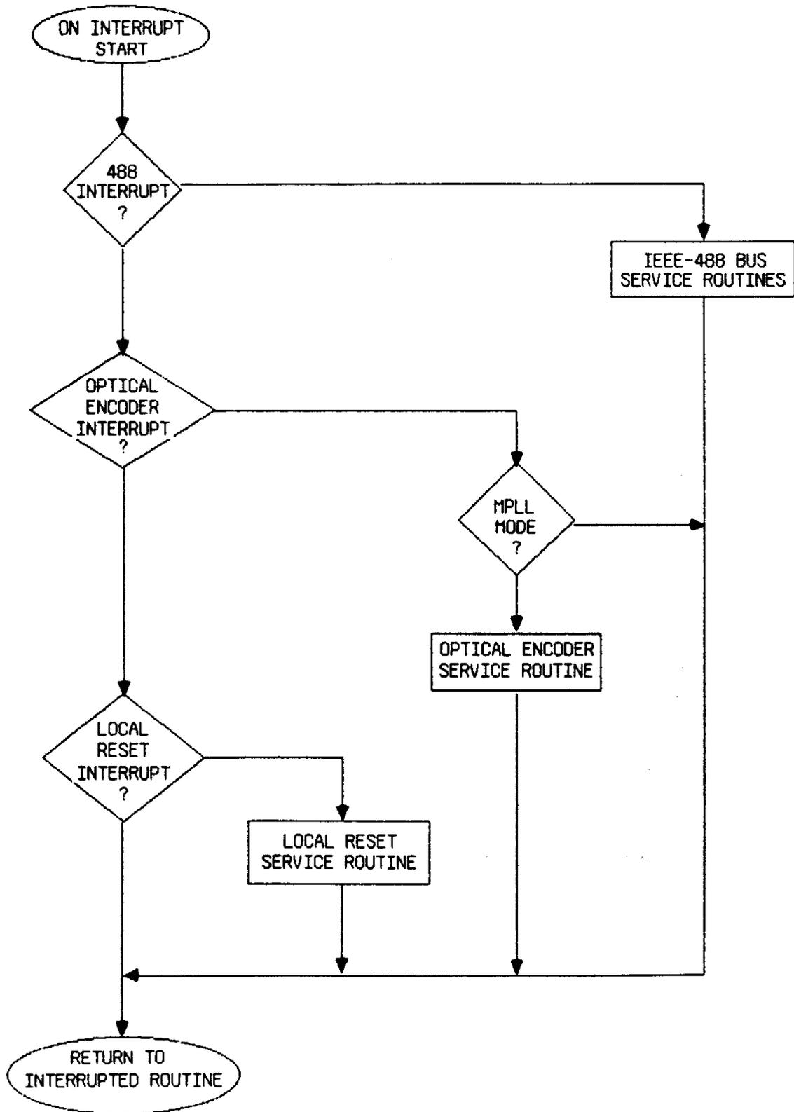
Figure 7. MPLL Interrupt Processing Flow
