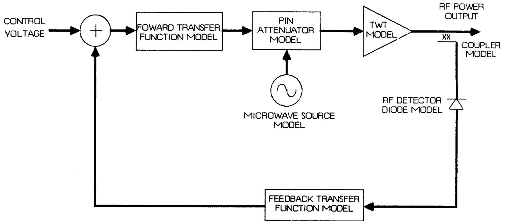
**Figure 9. MPLL Closed-Loop Dynamics Simulation Block Diagram**
