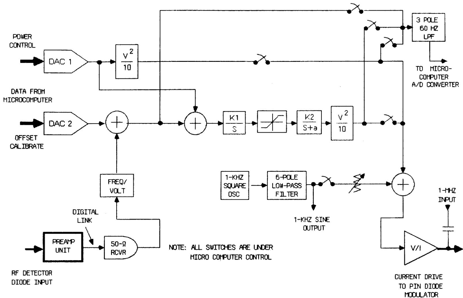
Figure 5. Analog Electronics Block Diagram
