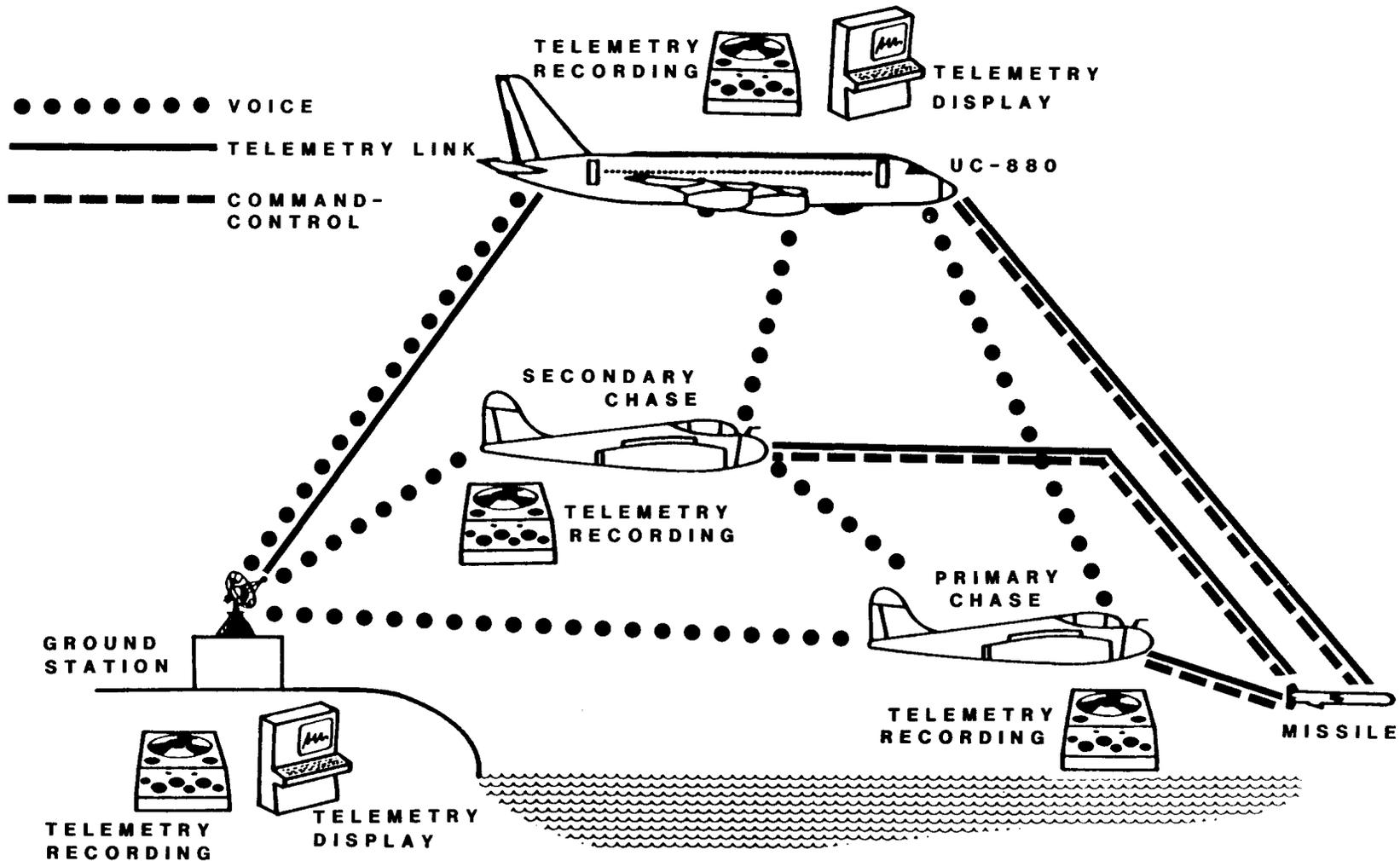
FIG. 4 TELEMETRY, COMMAND/CONTROL, AND COMMUNICATION LINKS
