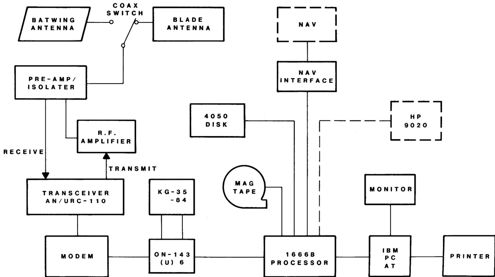
**FIG. 6 USQ-81V SYSTEM UC-880 INSTALLATION**
