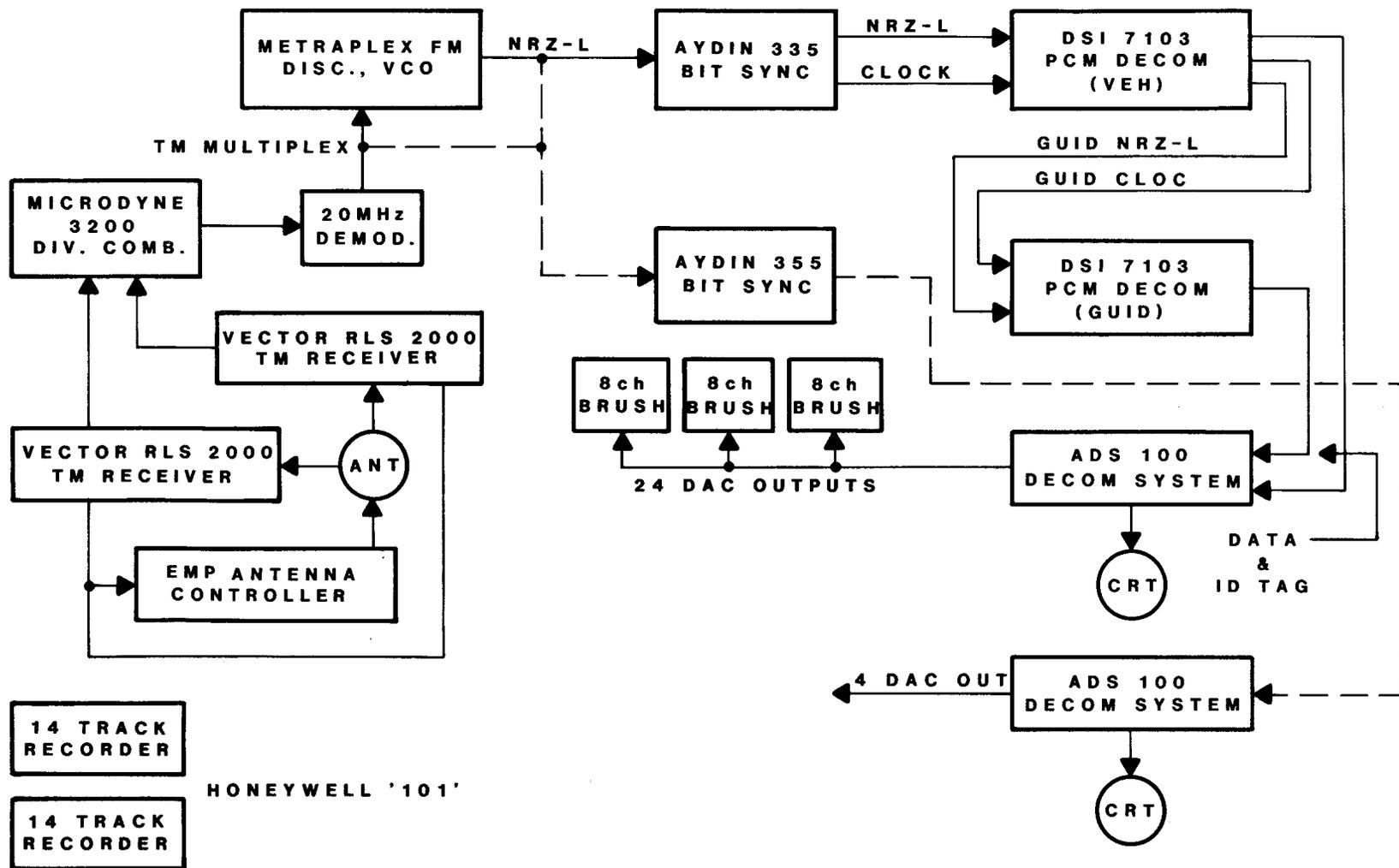
FIG. 5 UC-880 DATA PROCESSING, DISPLAY, AND RECORDING SYSTEM
