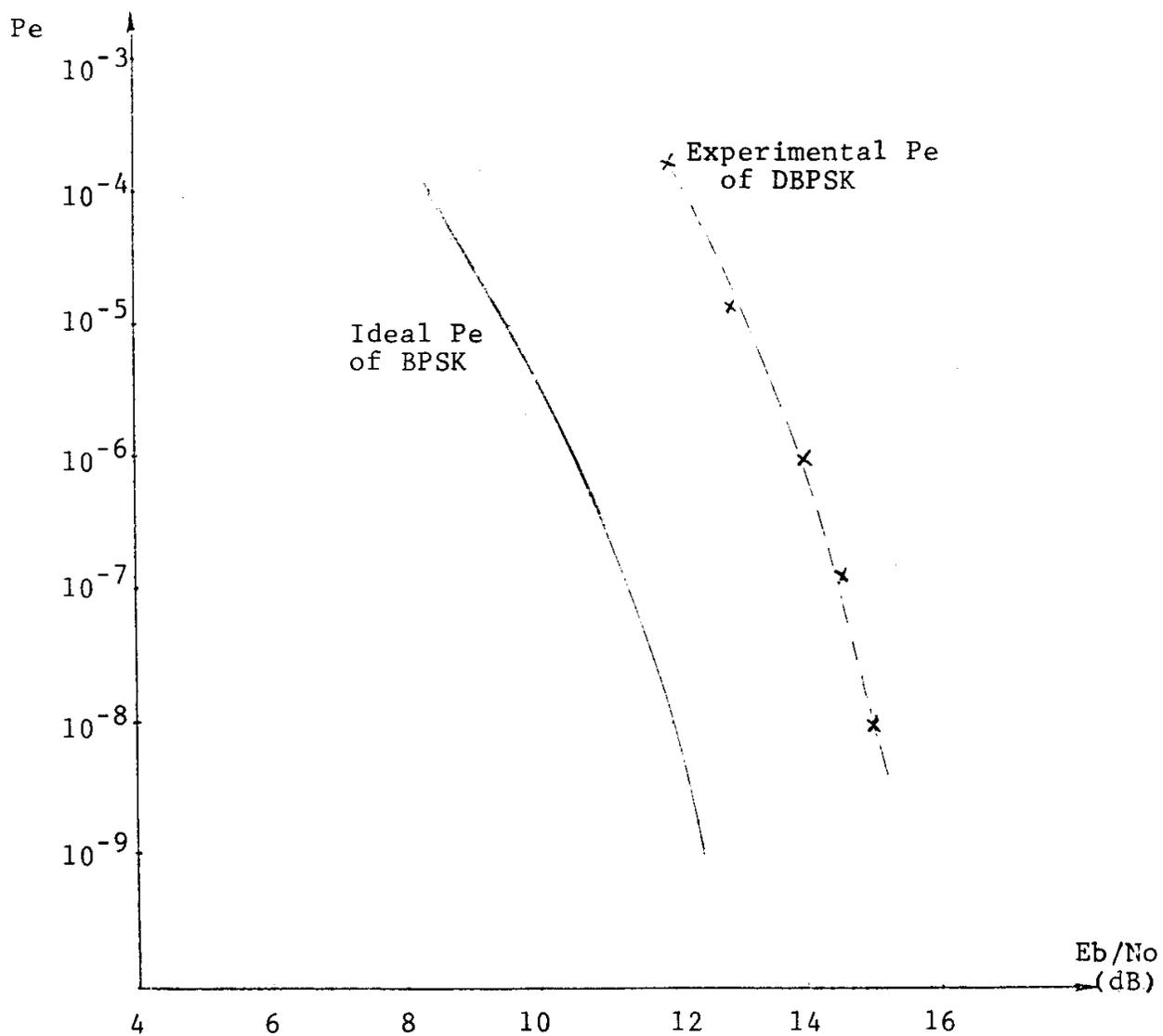
**Fig. 6 Probability of bit error  $P_e$  for experimental DBPSK modem**
