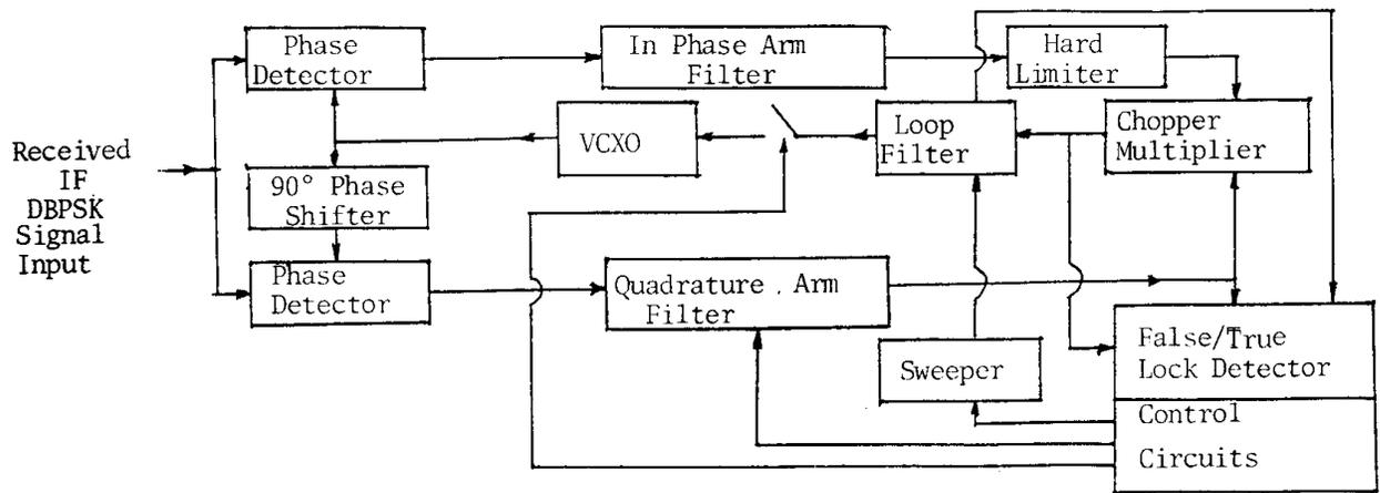
**Fig. 2 Costas Loop & Acquisition Aid Circuits**
