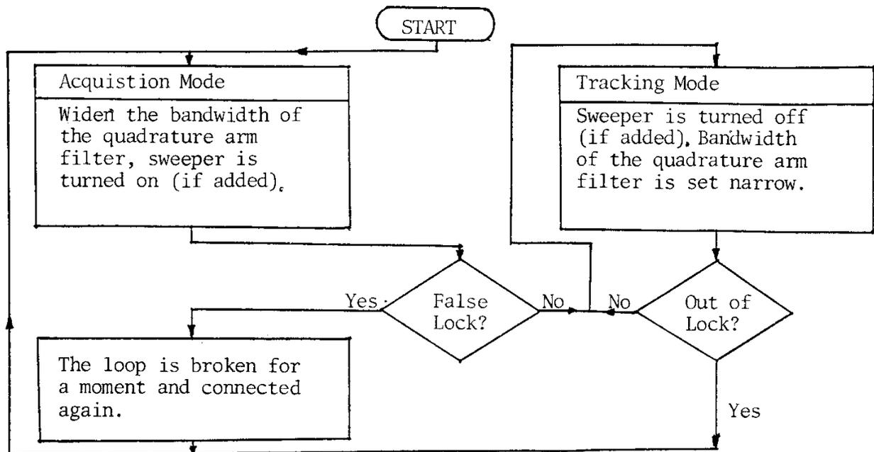
**Fig. 3 Flowchart of Loop's Operation Algorithm**
