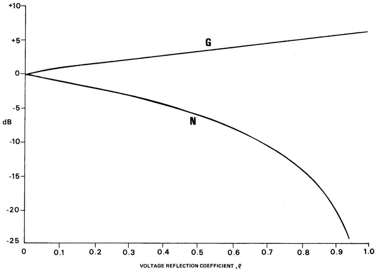
**Figure 2 - Gain & Null Depth for Reflective Surfaces**
