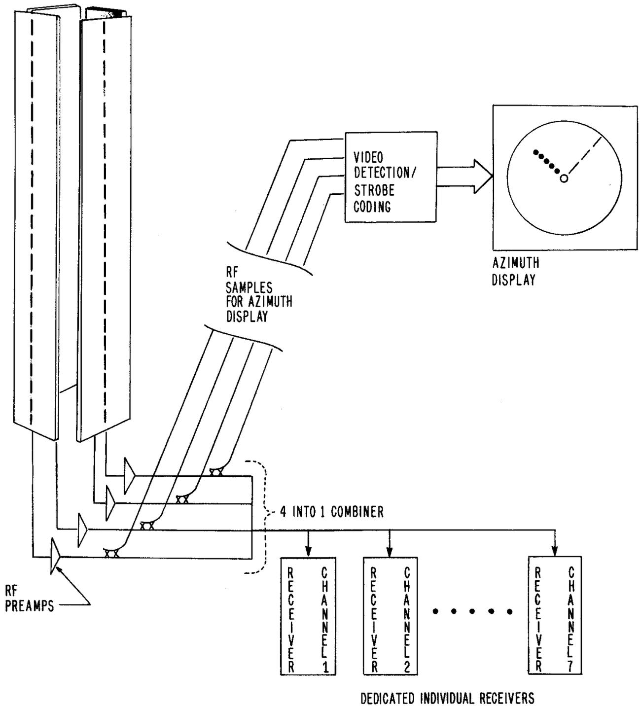
**Figure 4 - System Functional Operation**
