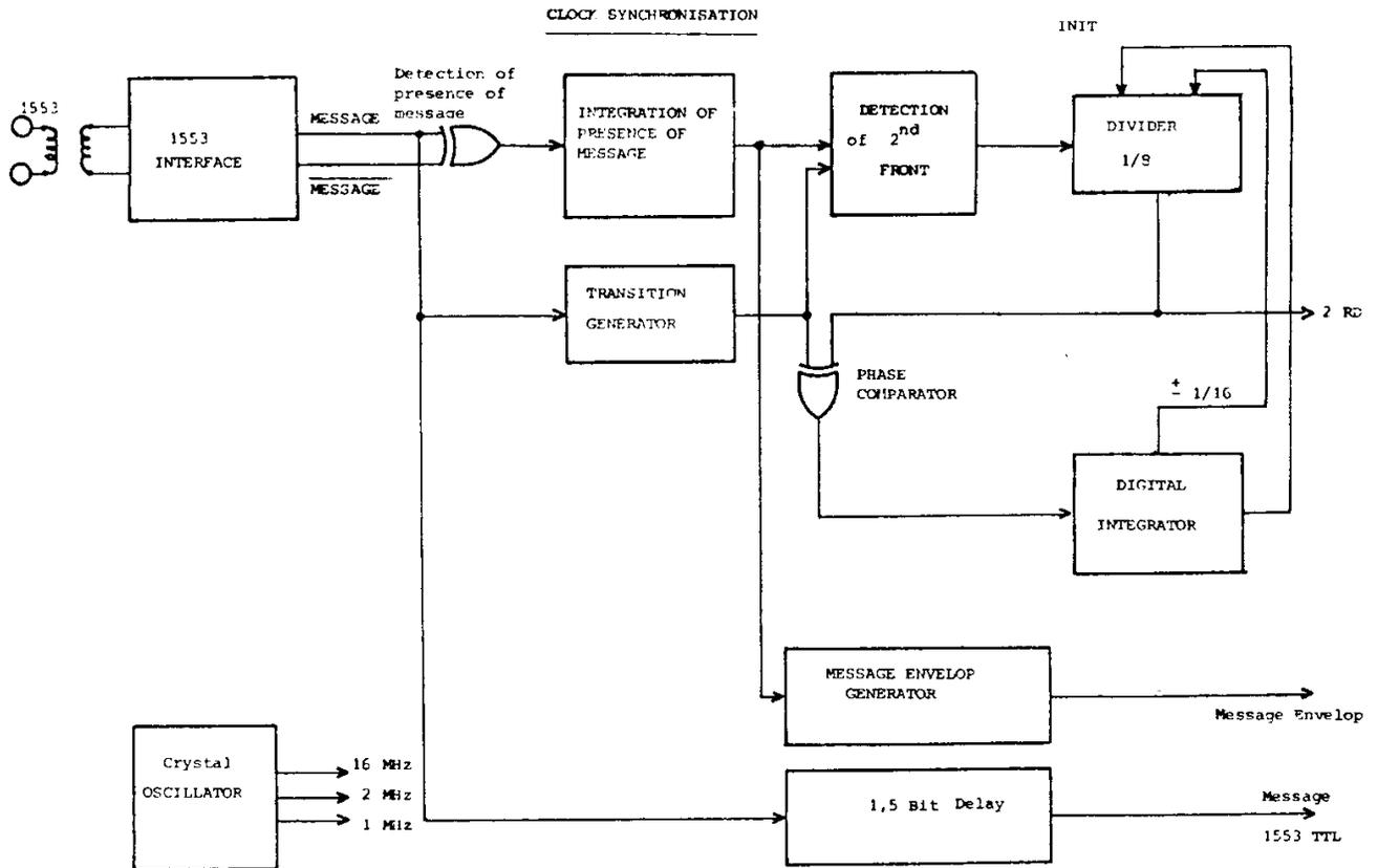
Ordinary standard circuits are not suitable, they reject the error words which is contrary to the “spy role” of the 1553 controller.
