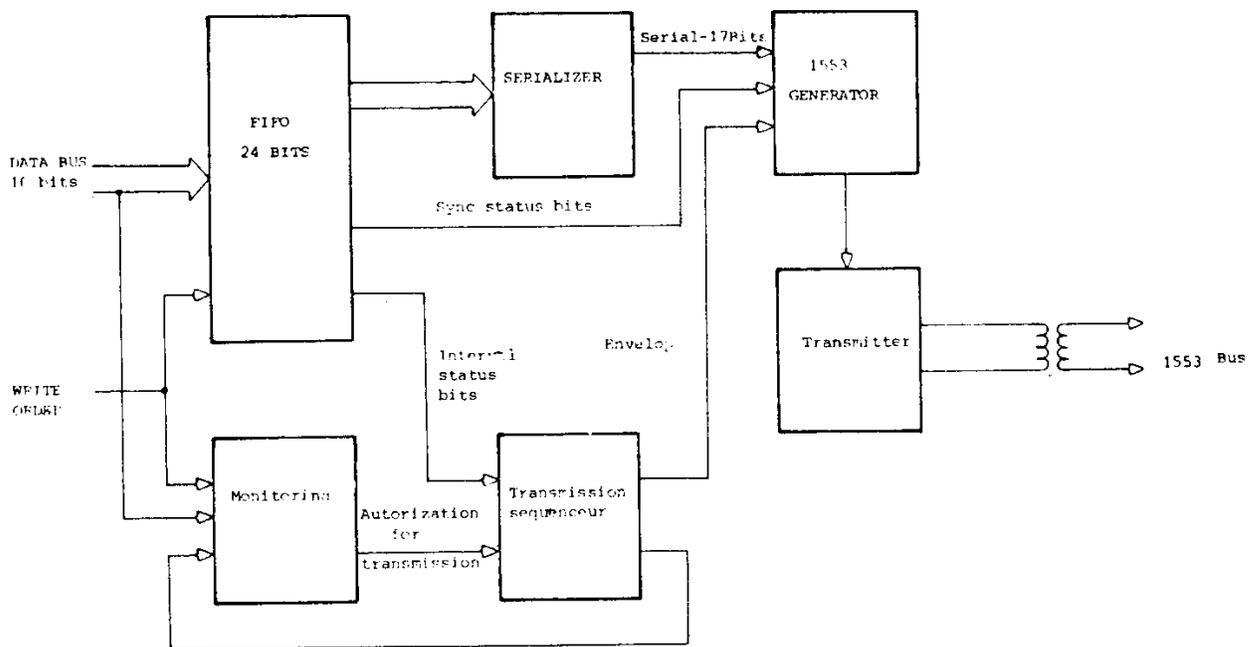
The duration of a 1553 word transmitted by telemetering is equal to 24 microseconds (3 bytes of 8 microseconds) minimum, in the case of a P.C.M. without parity.
