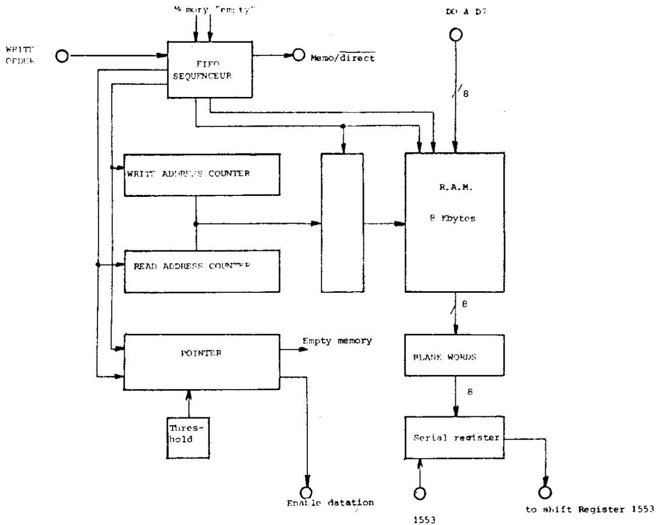
The addresses are supplied by the multiplexing of the states of two counters, one responsible for write addresses and the other for read.
