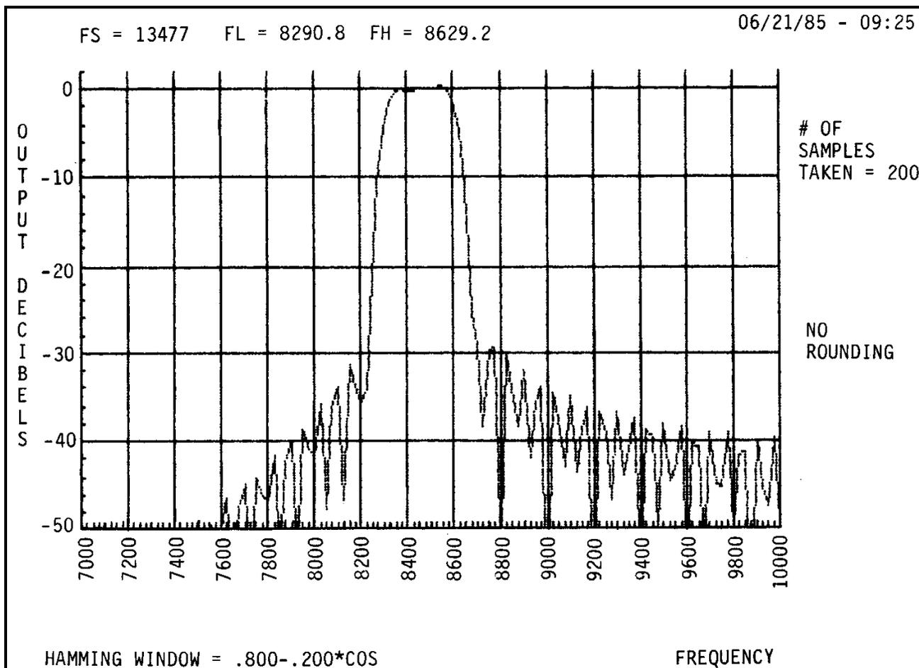
**Figure 2. IRIG Channel 2 Filter Response with Hamming Window**
