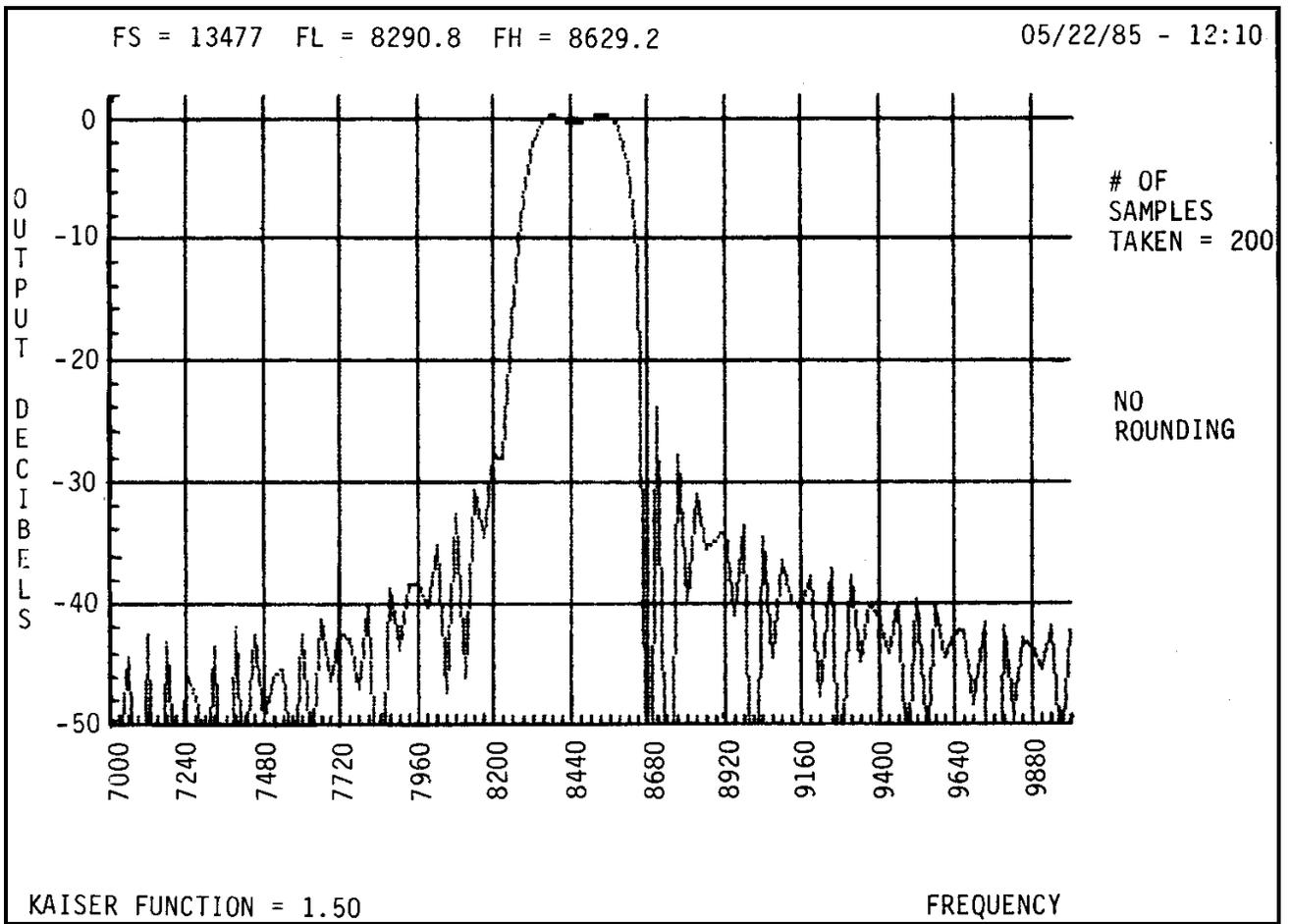
**Figure 3. IRIG Channel 2 Filter Response with Kaiser Window**
