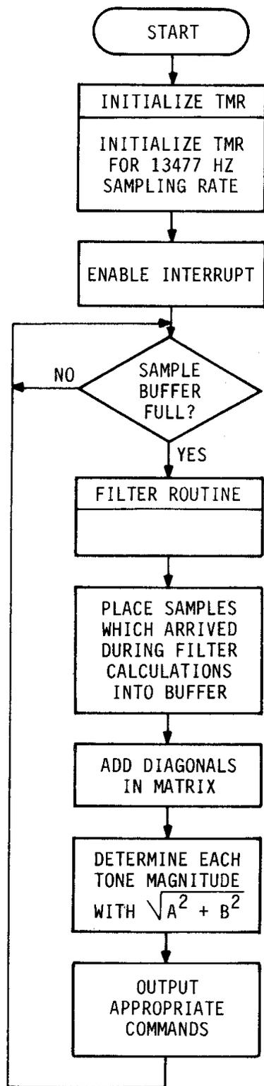
Figure 4. Top Level Signal Processing Flowchart
