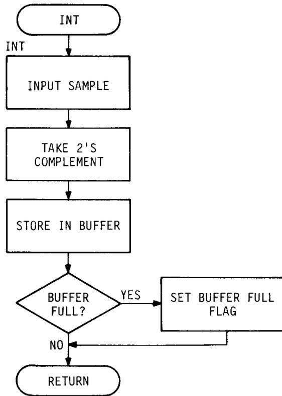
**Figure 5. Interrupt Routine Flowchart**
