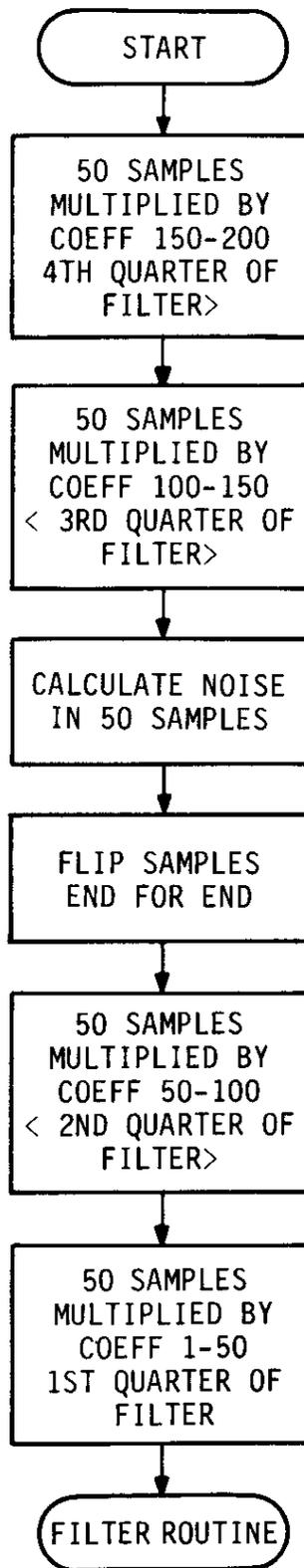
**Figure 6. Filter Routine Flowchart**
