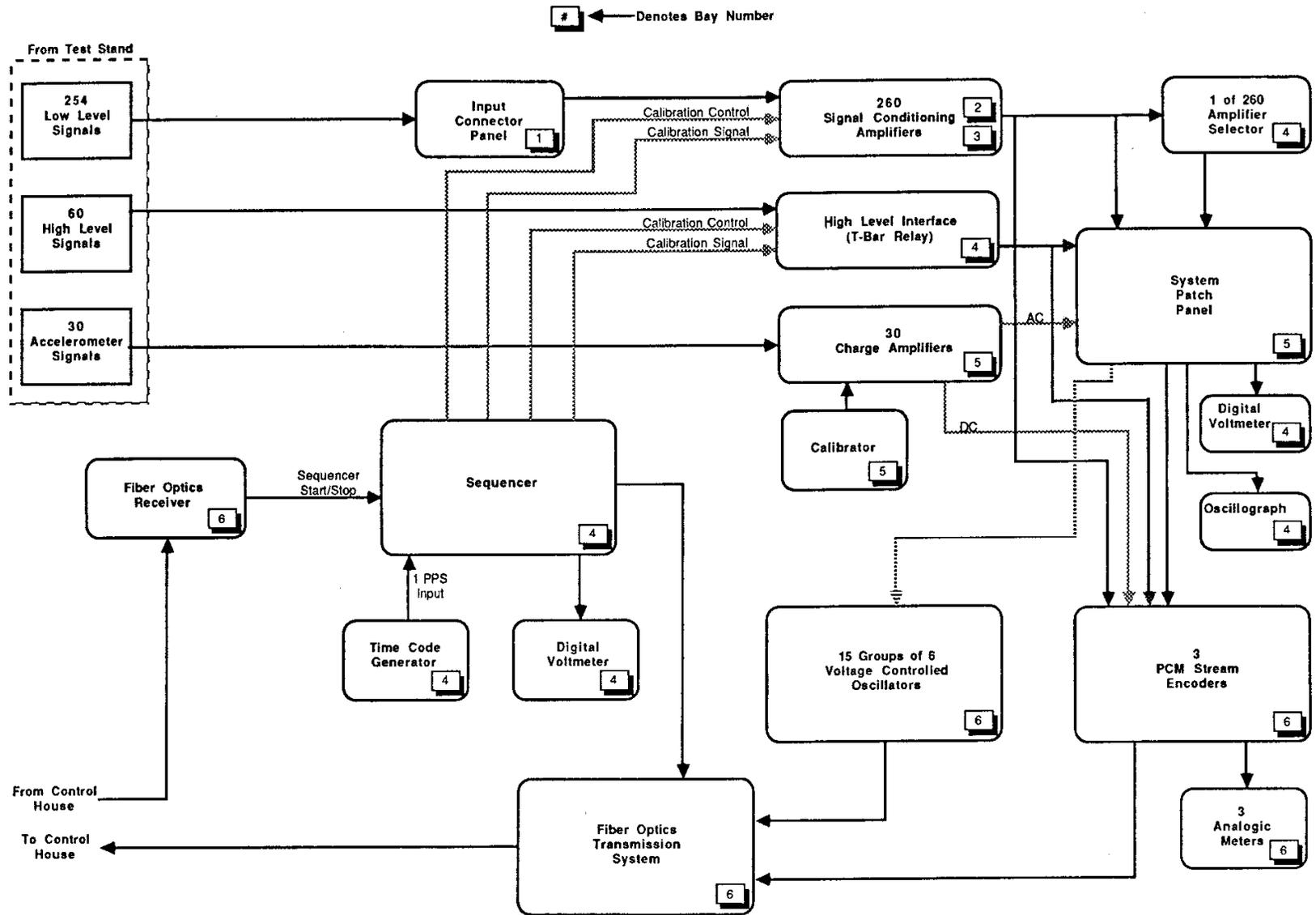
**Figure 1-1 - Instrument House Assemblies**
