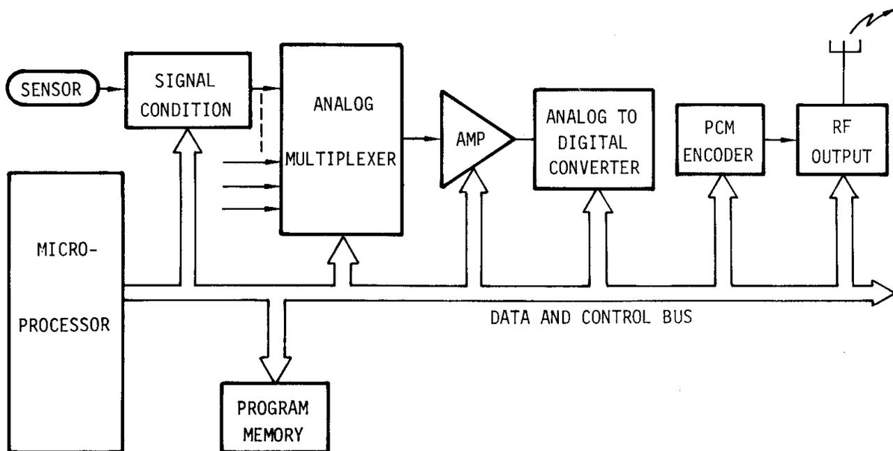
**FIGURE 3. PROGRAMMABLE TELEMETRY SYSTEM**
