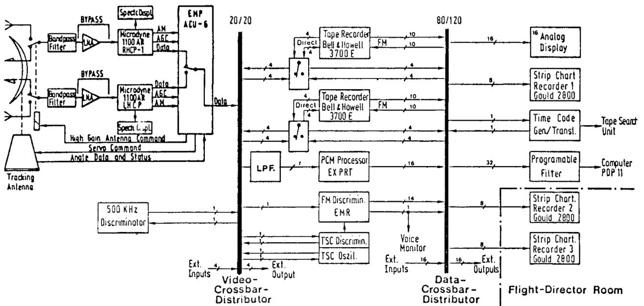
**Fig. 10 Telemetry-Ground Station**
