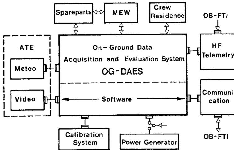
**Fig. 9 Schematic of On-Ground Flight Test Instrumentation**
