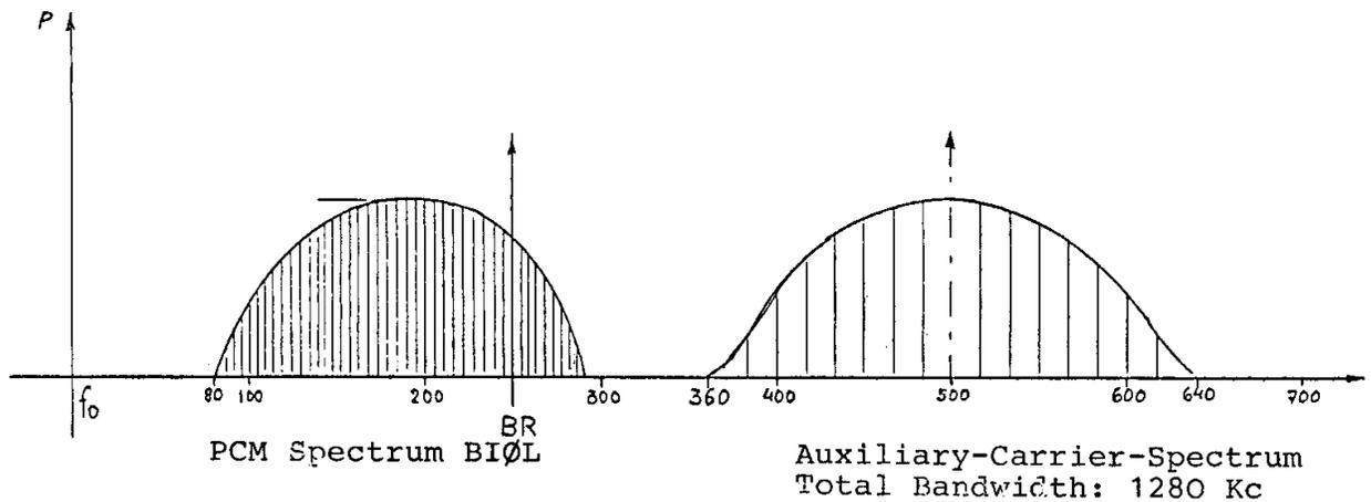
**Fig. 7 Frequency Spectrum PCM and 500 kHz Auxiliary Carrier**
