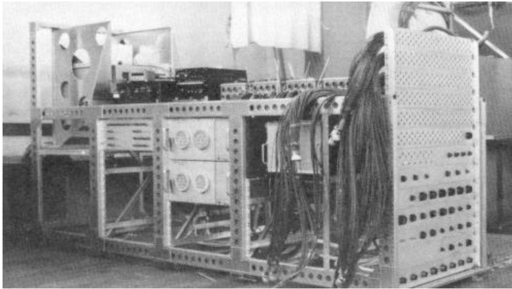
**Fig. 3 Rack-mounted OB-DAS for CN235 Aircraft**
