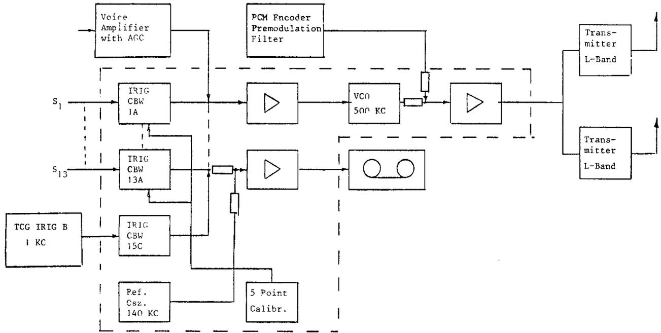
**Fig. 6 Airborne FM Telemetry Blockdiagram with Time Code IRIG B**
