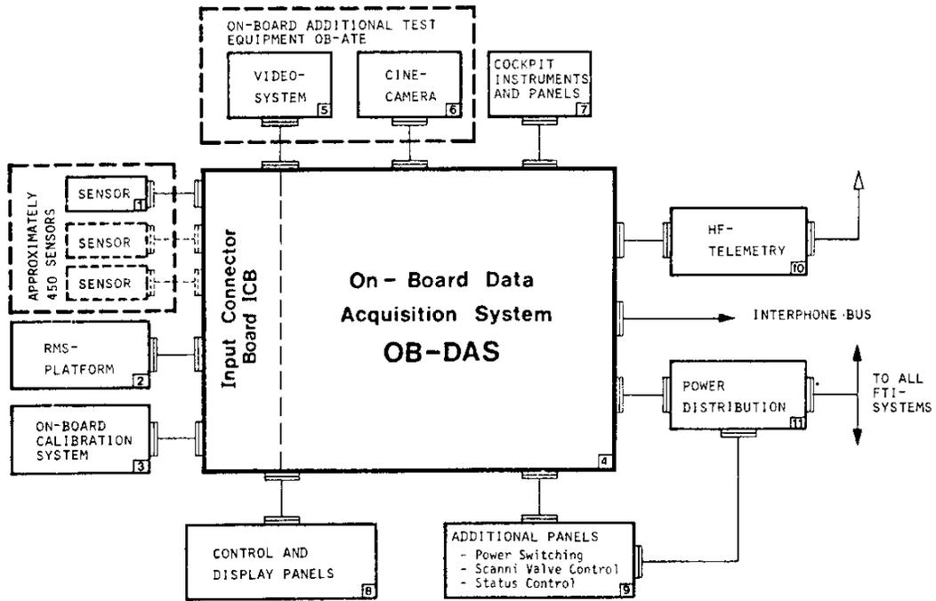
**Fig. 2** Schematic of On-Board Flight Test Instrumentation (OB-FTI)
