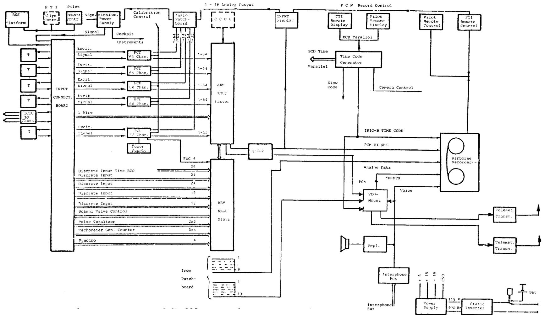
**Fig. 8 Blockdiagram of CN 235 On Board Data Acquisition System**
