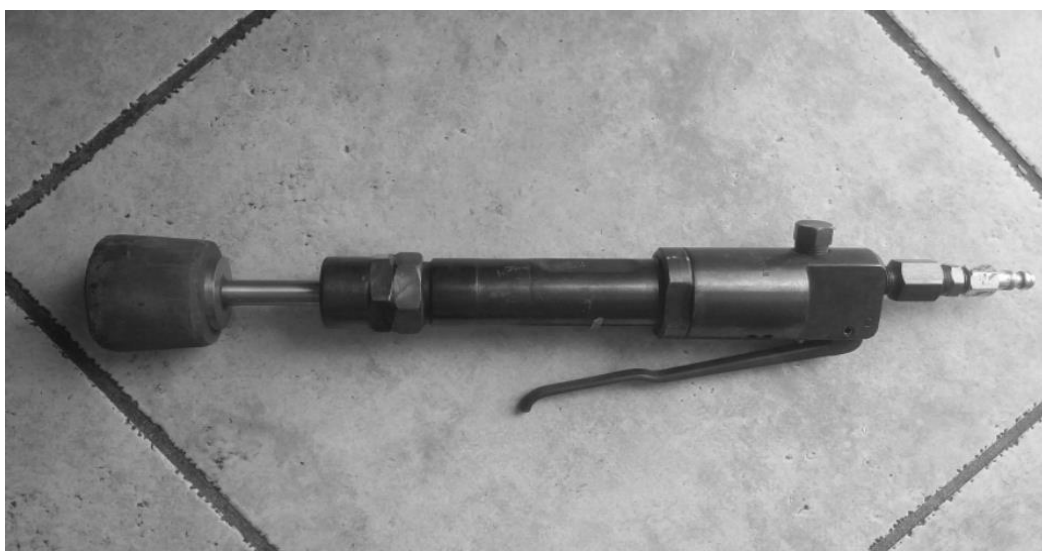
Figure 1: A sand rammer used to compact sand around a pattern at a foundry
