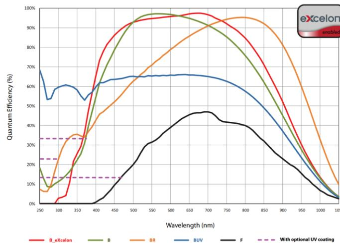
Figure 2.3. Plot of the quantum efficiency of PIXIS 2048B. The plot is labeled green. Retrieved from [http://www.princetoninstruments.com/userfiles/files/assetLibrary/Datasheets/Princeton\\_Instruments\\_PIXIS\\_2048\\_eXcelon-N5\\_1-10\\_22\\_14.pdf](http://www.princetoninstruments.com/userfiles/files/assetLibrary/Datasheets/Princeton_Instruments_PIXIS_2048_eXcelon-N5_1-10_22_14.pdf)
