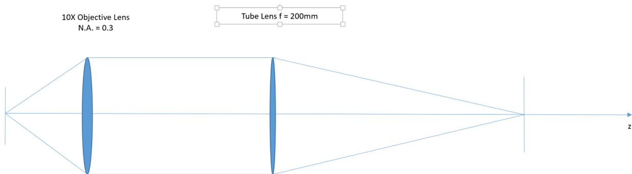
Figure 3.2. The lateral magnification of the objective lens and tube lens to acquire the N.A. in image space
