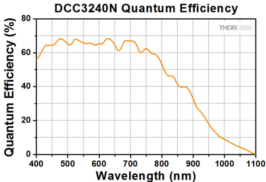
Figure 2.5. Plot of quantum efficiencies of DCC 3240N. Retrieved from [https://www.thorlabs.com/newgrouppage9.cfm?objectgroup\\_id=4024&pn=DCC3240N](https://www.thorlabs.com/newgrouppage9.cfm?objectgroup_id=4024&pn=DCC3240N)
