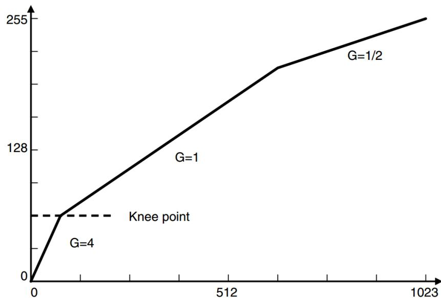
Figure 2.6. The mapping plot converting 10-bit data to 8-bit data. Retrieved from [http://www.e2v.com/content/uploads/2014/02/DSC\\_EV76C661.pdf](http://www.e2v.com/content/uploads/2014/02/DSC_EV76C661.pdf)
