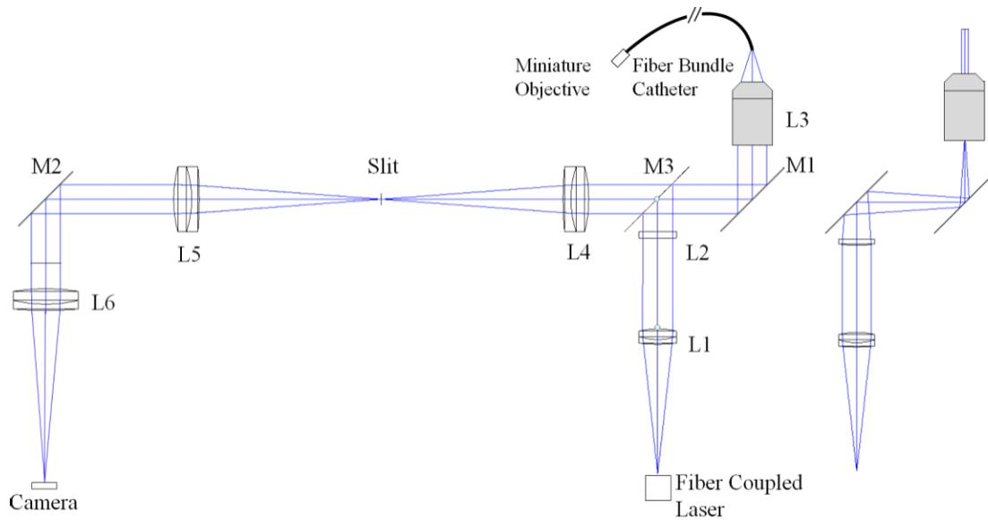
Figure 2.4. Diagram of OSU. Courtesy of T. Wu (2015)
