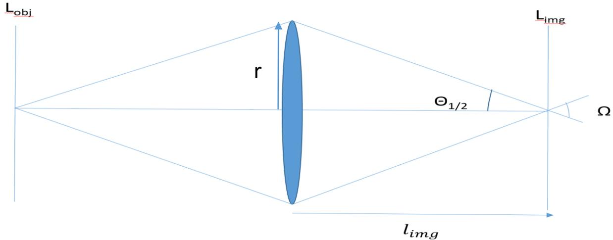
Figure 3.1. Simple optical system depicting the solid angle
