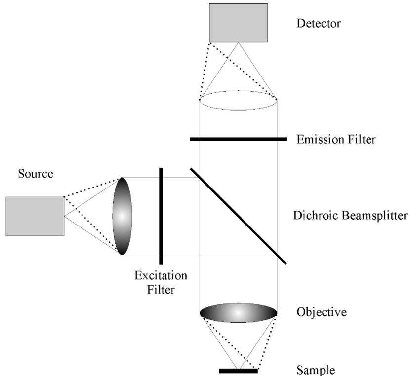
Figure 2.1. Conventional fluorescence microscope. Diagram courtesy of A. Rouse (2004)
