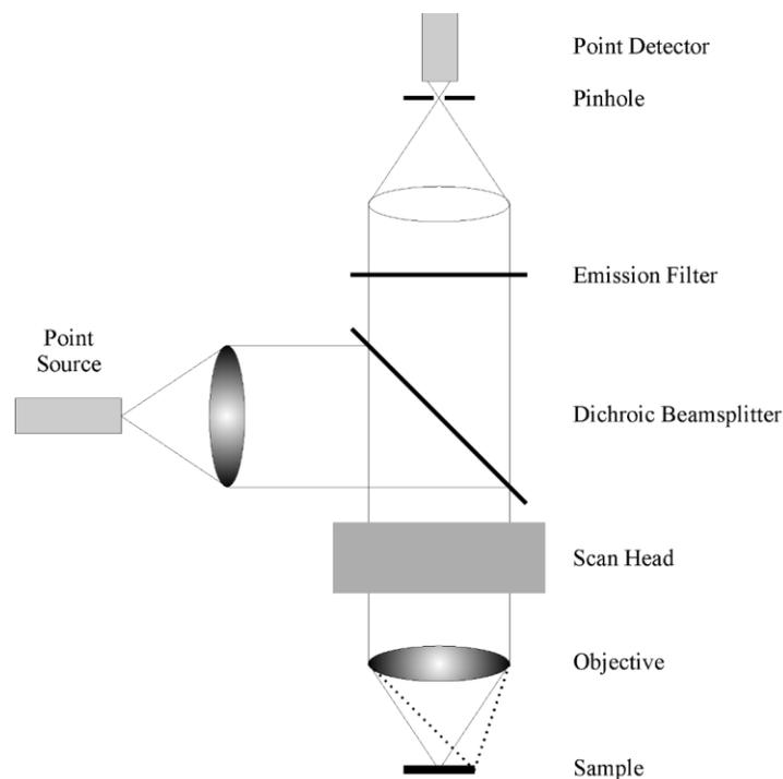
Figure 2.2. Conventional scanning confocal microscope. Diagram courtesy of A. Rouse (2004)
