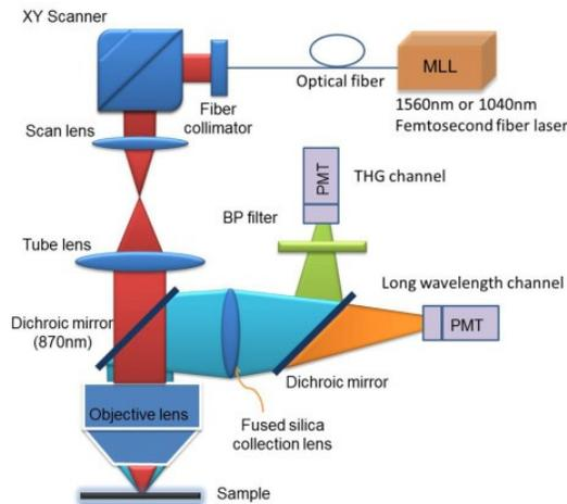
Figure 1. Block diagram of the MPM system used in this study.
