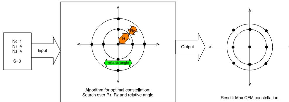
Fig. 2. Optimal constellation design algorithm for non-uniform signaling scheme.
