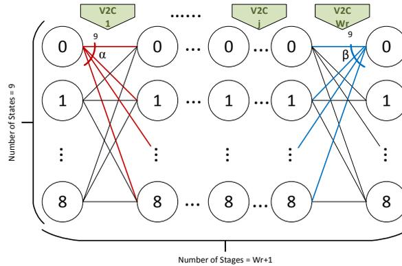
Fig. 6. Trellis graph of the BCJR algorithm-based check-node processor.
