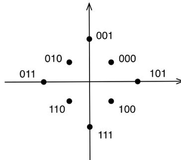
Fig. 4. The mapping rule for star 8-QAM.
