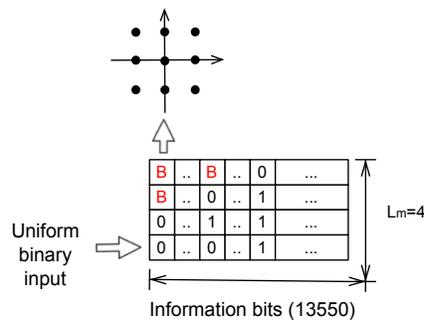
Fig. 8. Interleaver structure of 9-QAM.
