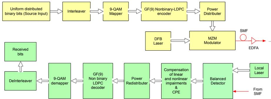
Fig. 7. Non-uniform 9-QAM coded modulation scheme based on nonbinary LDPC coding.
