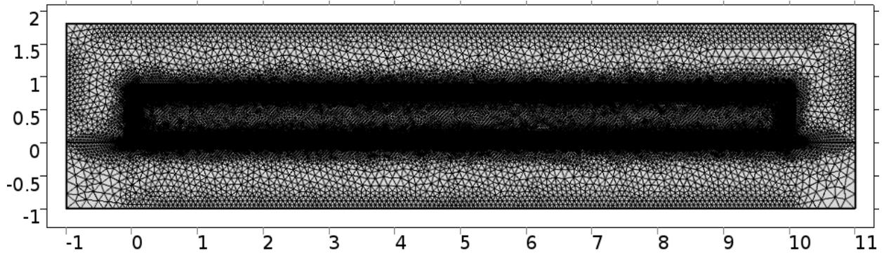
**Fig. S3.** The entire domain was meshed by free triangular. Total number of elements: 53,087.
