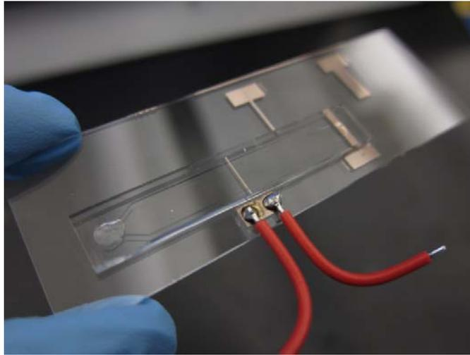
**Fig. S1.** An assembled PDMS microchannel with integrated parallel electrodes for investigating the long range electrothermal fluid motion.
