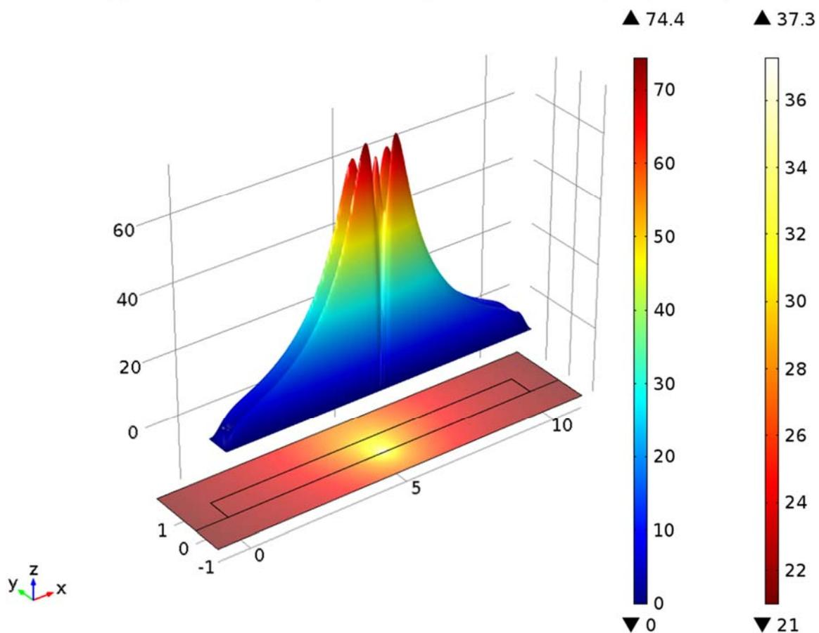
**Fig. S4.** Velocity and temperature profiles in an 800  $\mu\text{m}$  channel with 1 MHz square wave with 7 V peak-to-peak. The units of fluid velocity and temperature are  $\mu\text{m/s}$  and  $^{\circ}\text{C}$ .
