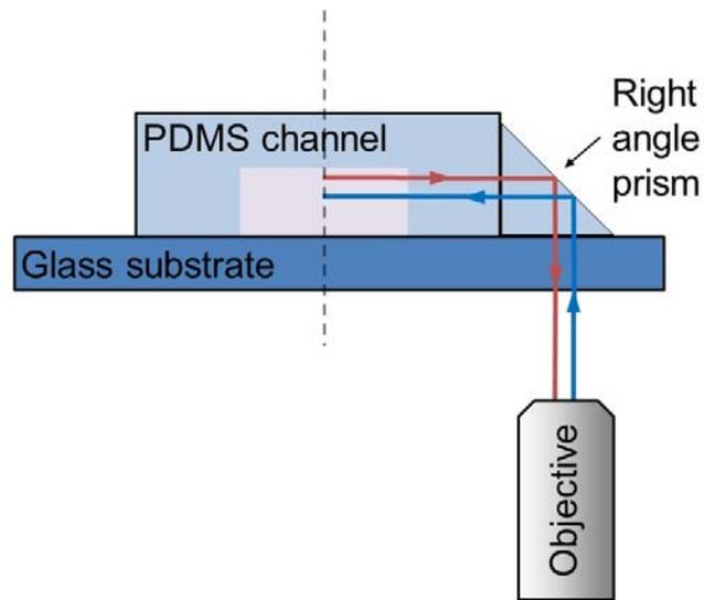
**Fig. S2.** Schematic illustration of the experimental setup for measuring the flow motion in the channel cross section. The dotted line indicates the focal plane.
