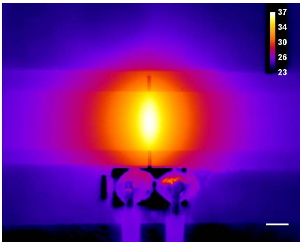
**Fig. S5.** The surface temperature of the PDMS channel measured by infrared thermometry. The channel height was 800  $\mu\text{m}$ . The voltage applied to the parallel electrode was 7V peak-to-peak voltage with 1MHz square wave.
