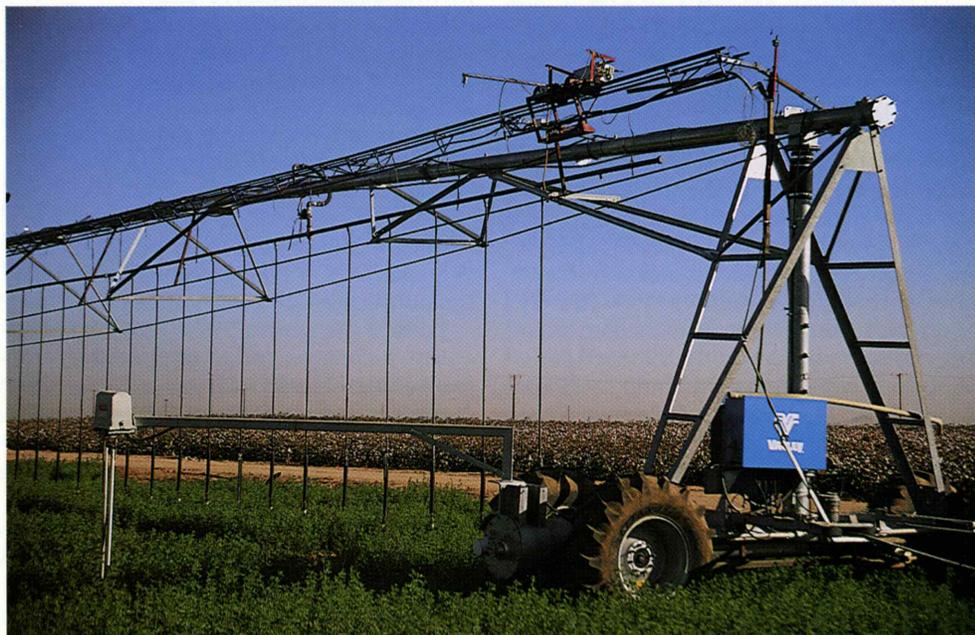
*The Agricultural Irrigation Information System (AGIIS) moves across the track mounted on top of a linear move irrigation system.*
