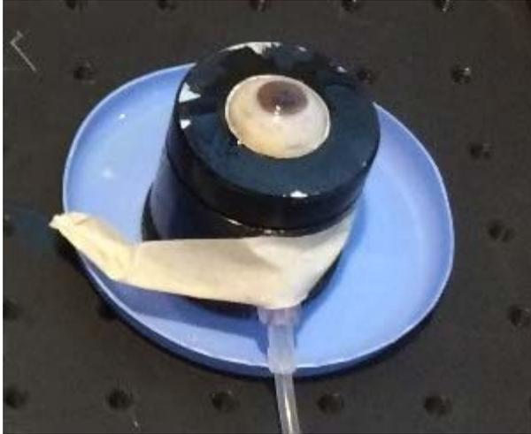
**Figure 4.** Ocular globe stabilizing apparatus for measuring IOP.
