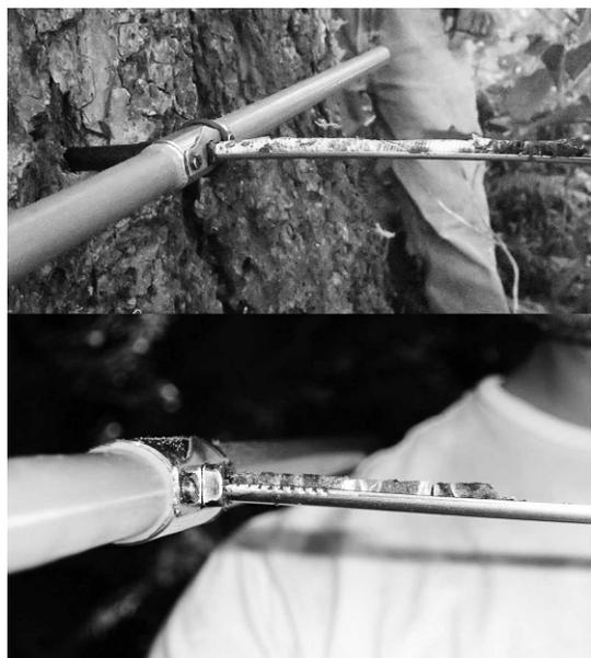
**Figure 2.** The results from not clearing the borer of problematic bark; note the twisted (rotated), mangled, debris-coated core (top). Bark being evacuated from the borer's shaft by means of the modified coring technique described in the methods (bottom).
