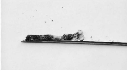
**Figure 1.** Compressed, gummy bark that was cleared from a jammed borer's shaft.
