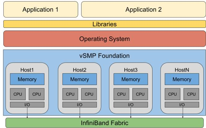
Fig. 1. vSMP System Expansion Mode
