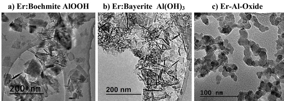
Figure 1. Ripening conditions for nanoparticle synthesis a.) 1 week 95 C b.) 1 week 160 C c.) 17 hours 160.
