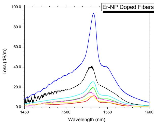
Figure 4. Erbium absorption peaks for NP-doped preforms.
