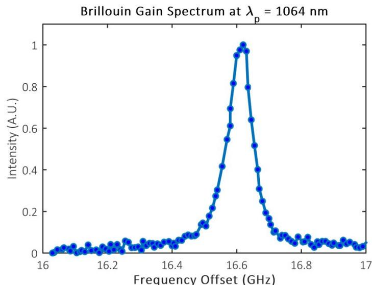
Figure 7. Brillouin gain spectrum for NP-doped fiber obtained from pump-probe experiment performed at 1064 nm
