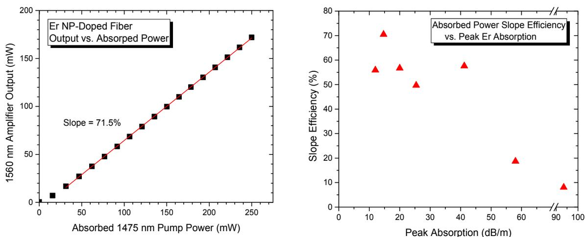
Figure 5. a.) MOPA output vs. absorbed pump power for an Er-NP-doped fiber, b.) slope efficiency for NP-doped preforms as a function of  $\text{Er}^{3+}$  absorption peak.
