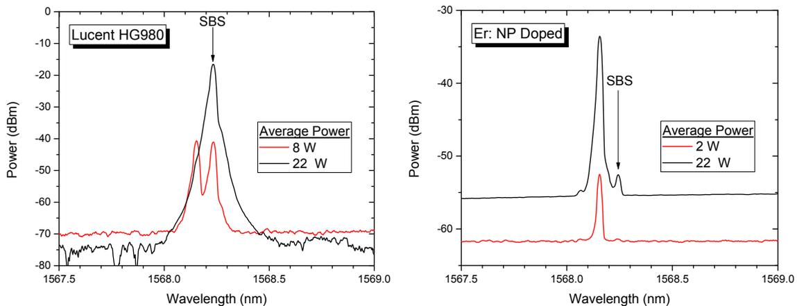
Figure 6. Backscattered Rayleigh and SBS peaks for a commercial fiber a.) and for NP-doped fiber b.)
