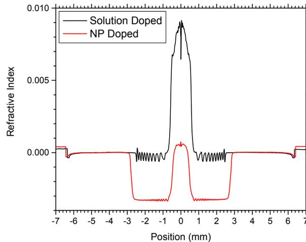
Figure 2. Refractive index profiles of preforms with NP- and solution-doped cores ( $\Delta n$  relative to silica)
