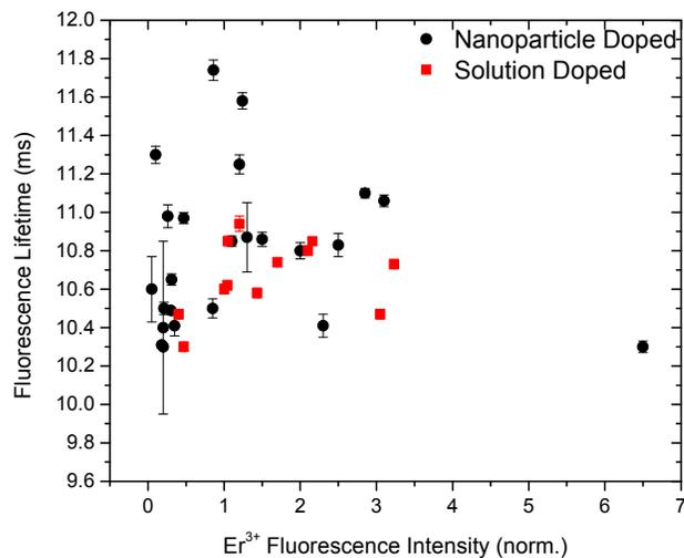
Figure 3. Fluorescence lifetime vs. intensity for NP-doped preforms and solution-doped preforms.
