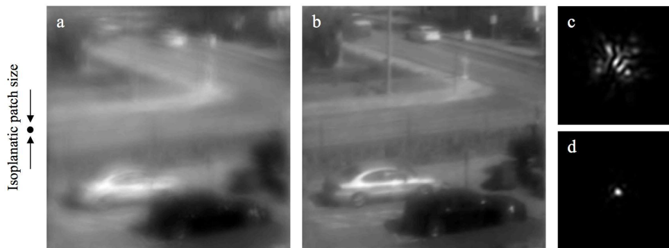
Figure 3. Examples of the simulated full-aperture images. With uncorrected atmospheric aberration (a); after correction (b). The on-axis PSFs for the two images are shown in (c) and (d), with different gray scales and expanded by a factor of four compared to the images. For reference, the size of the isoplanatic patch is shown on the left.
