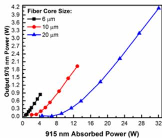
Fig. 2. Output powers of the 976 nm fiber amplifiers as a function of 915 nm absorbed power.
