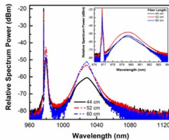
Fig. 3. Optical spectra of the 6  $\mu\text{m}$  core fiber amplifiers with different fiber lengths (resolution: 0.1 nm). Inset: spectra of 0.01 nm resolution.
