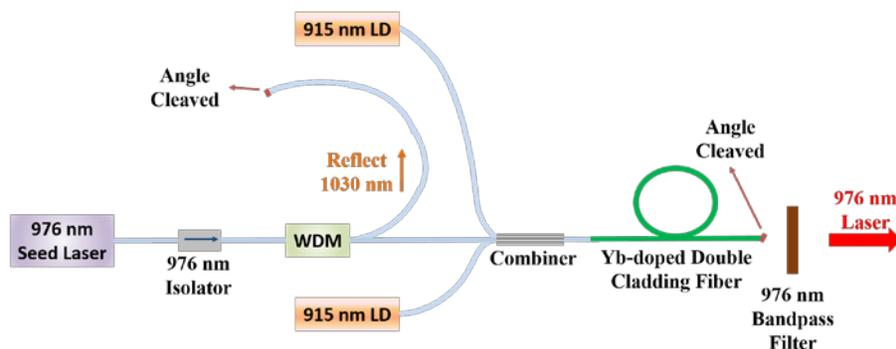
Fig. 1. Experimental setup of a 976 nm Yb<sup>3+</sup>-doped fiber amplifier.
