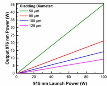
Fig. 4. Calculated output powers of the 976 nm fiber amplifiers as a function of the 915 nm launch power for fibers with different cladding diameters.
