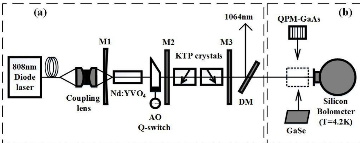
Figure 1. Experimental setup for THz DFG system. (a) is the part of dual-wavelength KTP OPO and (b) is the part of THz generation based on QPM-GaAs/GaSe crystals.
