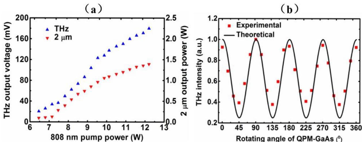
Figure 3. (a) THz output voltage and 2- $\mu\text{m}$  output versus LD pump power; (b) Normalized THz output voltage while rotating QPM-GaAs in the (110) plane.
