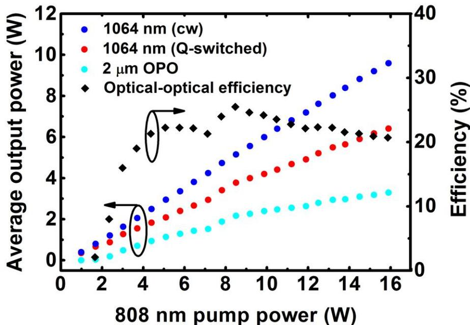
Figure 2. Output characteristics of the Nd:YVO<sub>4</sub> laser and KTP OPO
