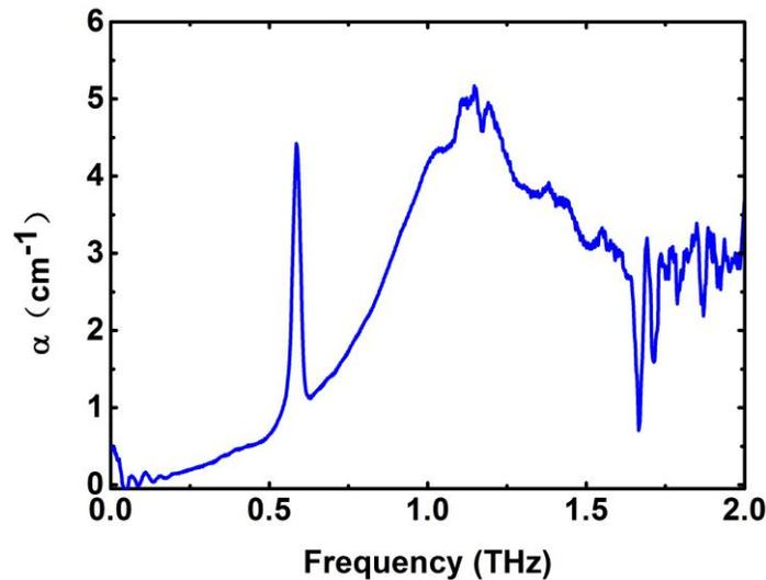
Figure 5. Absorption coefficient for the 15 mm-long GaSe crystal in the experiment
