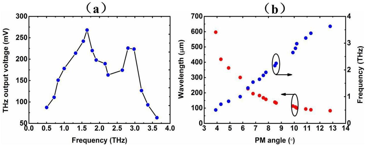
Figure 4. (a) THz output voltage at different frequencies; (b) THz wavelength and frequency versus the PM angle.
