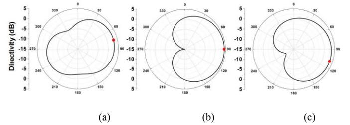
Fig. 4 2D directivity patterns in the  $zx$ -plane when the angle between the two OFF diodes is varied: (a)  $100^\circ$ , (b)  $120^\circ$ , and (c)  $140^\circ$ , while the other design parameters remain fixed. The main-beam direction is indicated as a red point in each sub-figure.
