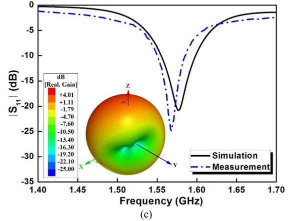
Fig. 7 The measured and simulated values of  $|S_{11}|$  (reflection coefficient values) as functions of the source frequency for the reconfigurable Huygens ESA in all three diode states, together with their corresponding simulated 3D radiation patterns at the resonance frequency 1.577 GHz. (a) State A, (b) State B, and (c) State C.
