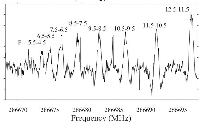
**Figure 3.** Millimeter/submillimeter direct absorption spectrum of the  $J = 9 \leftarrow 8$  rotational transition of  $^{49}\text{TiO} (X^3\Delta_2)$  near 286 GHz in the  $\Omega = 2$  ladder only. At the lower frequency, the hyperfine octet is distinct, but the spacing between lines decreases with decreasing  $F$  quantum number (see Figure 2). This spectrum was generated in a single scan of 70 s with a width of 30 MHz.
