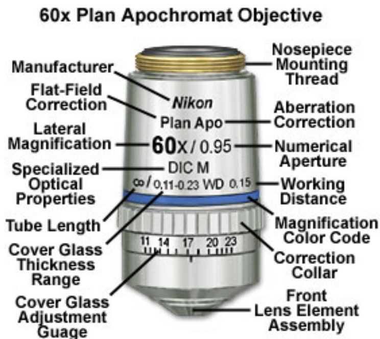
Figure 2.1 Objective Markings of a 60x Plan Apochromat Objective.
