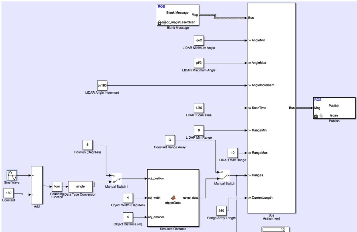
Figure 6 – LIDAR Simulator ROS Node.
