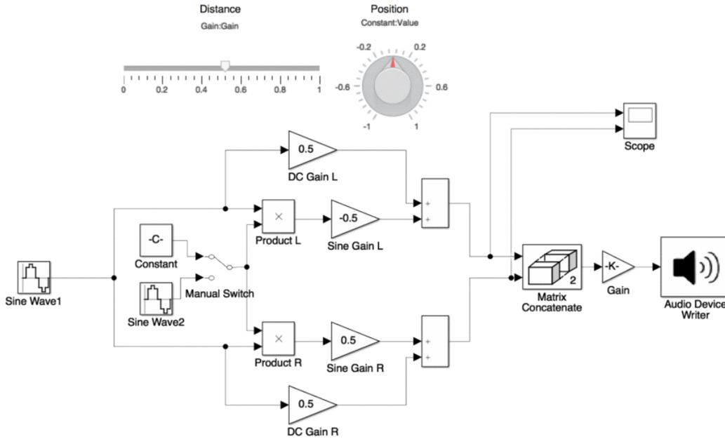
Figure 5 – Audio Generation MATLAB Simulation.
