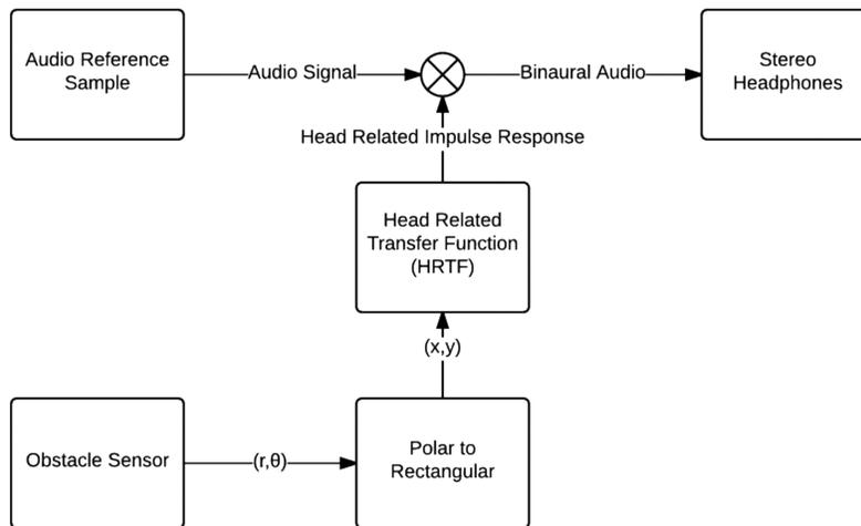
**Figure 4 – Audio Processing Block Diagram.**
