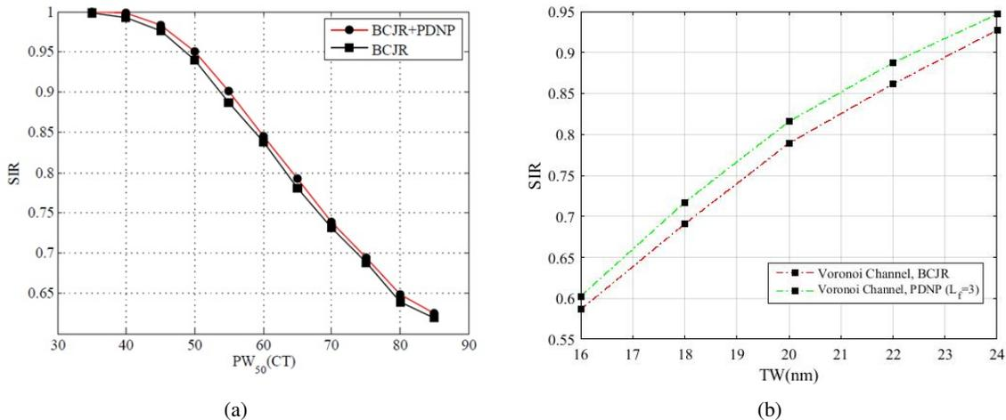
Fig. 2. Investigating the performance gain obtained of using the PDNP in computing the SIR using the forward recursion BCJR. (a) shows the variations of SIR vs. ITI. By increasing  $PW_{50}(CT)$ , ITI is increased since the reader senses more from two neighboring tracks. (b) shows SIR vs. TW.
