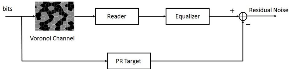
Fig. 1. The block diagram of TDMR system including read channel and equalizer is given. A simplified read channel architecture where the readback signal from the medium is equalized to achieve a controlled ISI called partial target response.
