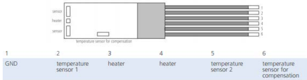
Figure 11: FS2 Thermal Mass Flow Sensor Layout and Pin Configuration
