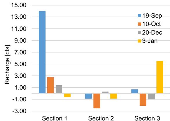
**Figure 9:** Select results from mass balance show negative recharge caused by inaccurate lag times applied to streamflow measurements
