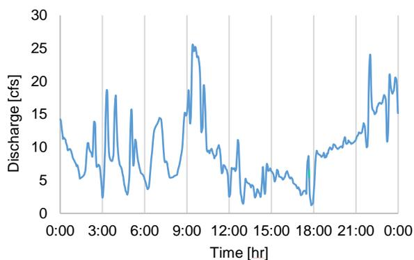
**Figure 5:** Reported outflow from Agua Nueva on 10/18/2016 showing high variability on small time frames
