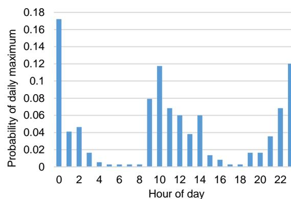
**Figure 6:** The histogram shows the probability of maximum discharge occurring during each hour of the day and reveals two daily peaks in outflow, at 10:00 a.m. and 12:00 a.m.
