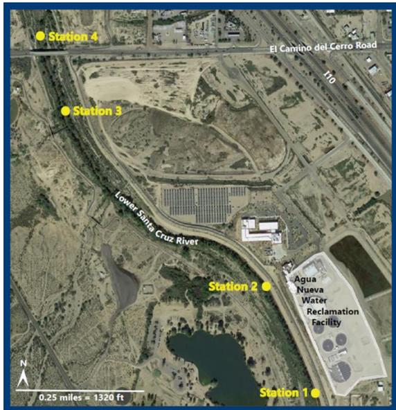
**Figure 3:** Overview of study area. Four monitoring stations were set up, beginning at the Agua Nueva outflow to the Santa Cruz River (Station 1) and spanning approximately 1 mile of channel length. The stations “bookend” three sections for recharge estimation.
