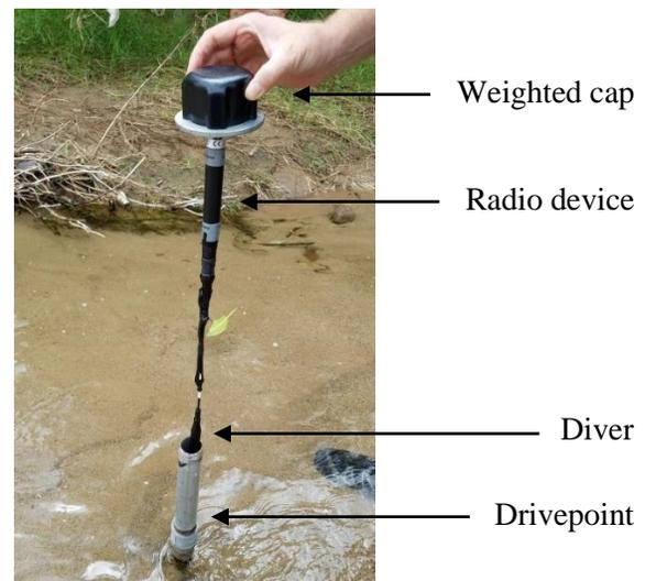
**Figure 4:** Diver being inserted into drivepoint installation at Station 2
