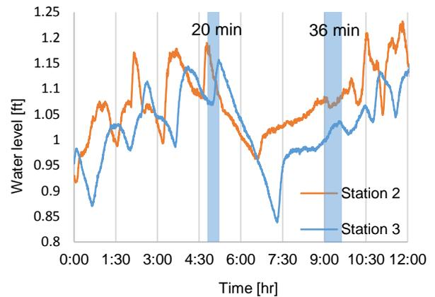
**Figure 8:** Water level at Station 2 and Station 3 show that travel time is dependent on river stage and varies depending on the level of the peak
