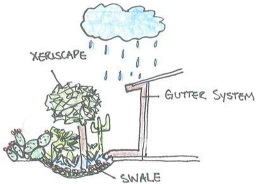
Figure 10 Example of Rainwater Harvesting Using Swales
