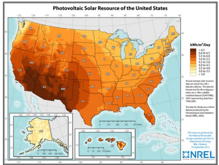
Figure 3. A map of peak sun hour values, measure in kilowatt hours per square meter per day. The higher the value, the longer sun is shining during a 12-hour period.
