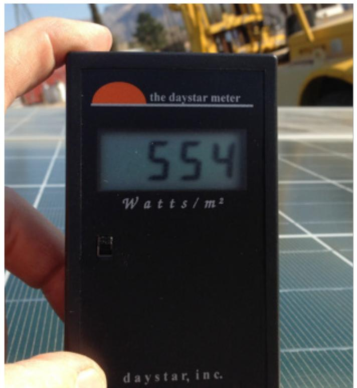
Figure 4. A solar irradiance meter (pyranometer) is used to measure the light intensity of the sun when the end of the meter is directed at the sun. Solar module power values are based on an irradiance level of 1,000 W/m<sup>2</sup>.
