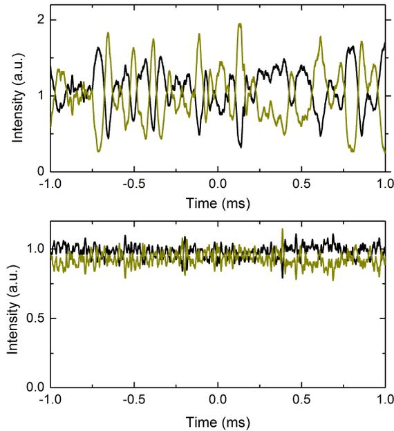
Figure 8: Fast photodiode readings of the two lasing bands for V-cavity (top) and F-cavity (bottom). The magnitude of the anti-correlation noise is indicative of the competition between the two modes.
