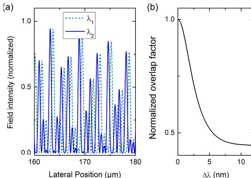
Figure 10: (a) Cross section of a simulated interference pattern for an F-cavity's intracavity field within the gain spot. (b) Plot of the overlap factor for two interference distributions based on their wavelength separation.
