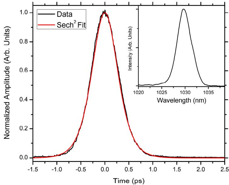
Figure 2: Autocorrelation of 410 fs pulse with (inset) corresponding 3nm spectrum.
