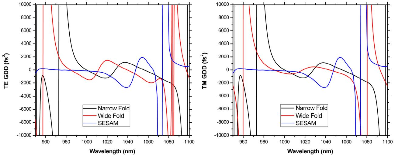
Figure 5: Simulation of single pass GDD in our VECSEL for narrow (black) and wide (red) angles, for both cavity TE mode (left) and cavity TM mode (right). Measured SESAM GDD (blue) is included in both for reference.
