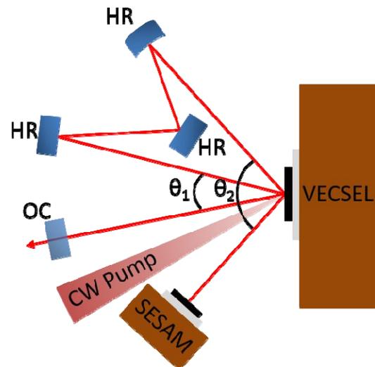
Figure 1: Schematic of an F-cavity designed for modelocking.
