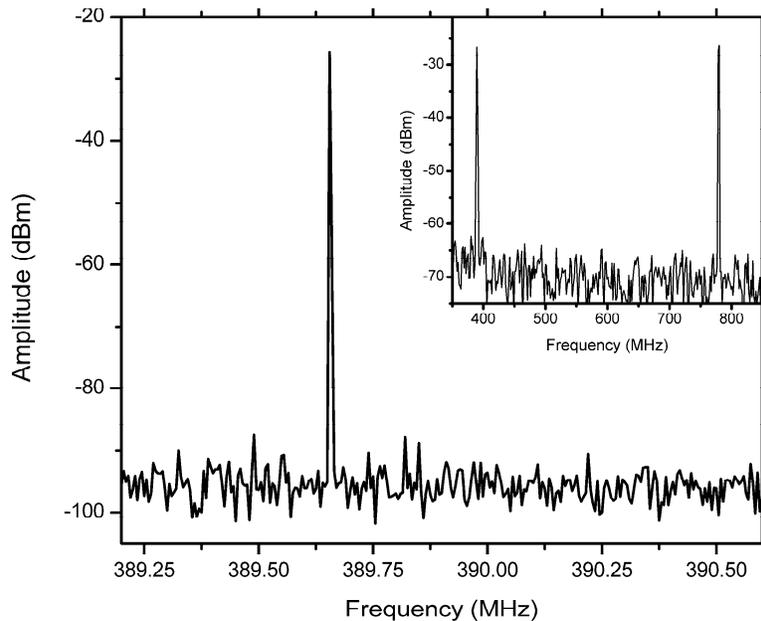
Figure 3: Recorded RF spectrum displaying narrow linewidth and (inset) lower resolution displaying first and second harmonics of the RF peak..
