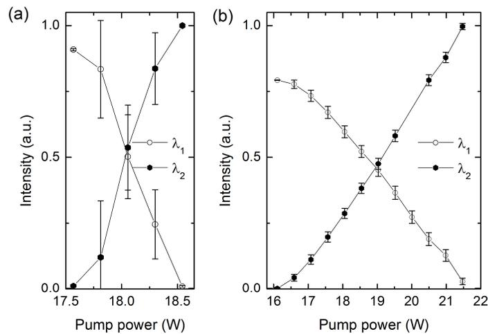
Figure 9: Operational ranges for stable 2-color emission in terms of pump power for (a) V-cavity and (b) F-cavity. Error bars indicate the magnitude of the noise behavior shown in Fig. 8
