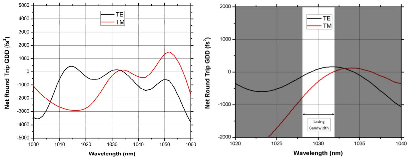
Figure 6: Simulated net roundtrip GDD for our VECSEL chip in our F-cavity design for cavity TE (black) and TM (red) modes. (Right) Zoom of this data displaying relevant details to the highlighted lasing bandwidth.
