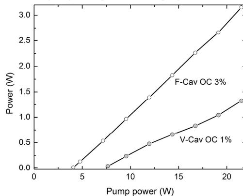
Figure 7: Power curves for F-cavity and comparison V-cavity. 2-color operation was stable for most of the F-cavity portion of this curve, but the maximum power with equal power in both modes was 2.6W.
