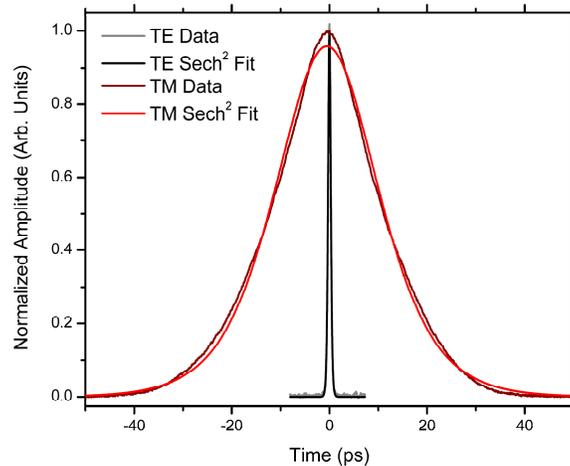
Figure 4: Pulse width comparison between operation when the cavity TE mode is enforced (black; see Fig 2 for zoom) and when its TM mode is enforced (red).
