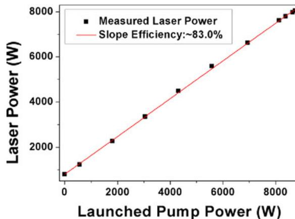
Fig. 6. The laser power output from the amplifier vs. launched pump power.
