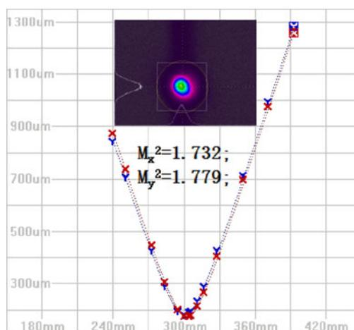
Fig. 4. The beam quality factor ( $M^2$ ) for the laser with 5010 W laser power. Inset: the typical laser beam profile.
