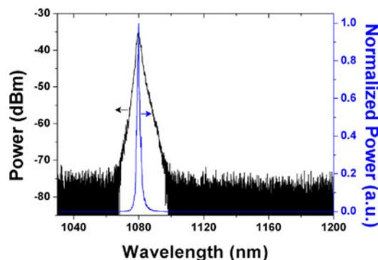
Fig. 7. The output spectrum for the amplified laser with a power of 8050 W.
