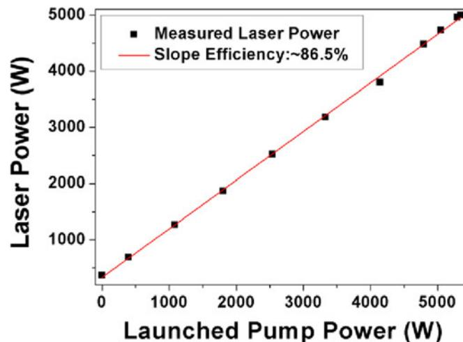
Fig. 2. The laser power output from the amplifier vs. launched pump power.
