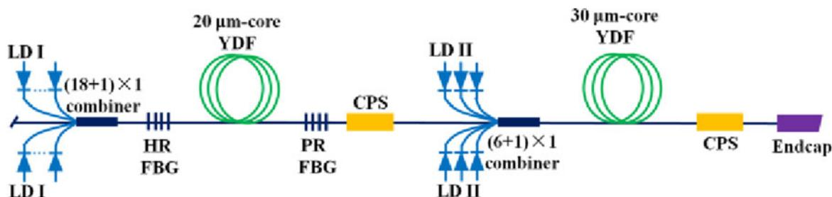
Fig. 1. Schematic configuration of the 5 kW near-diffraction-limited cw monolithic fiber laser.
