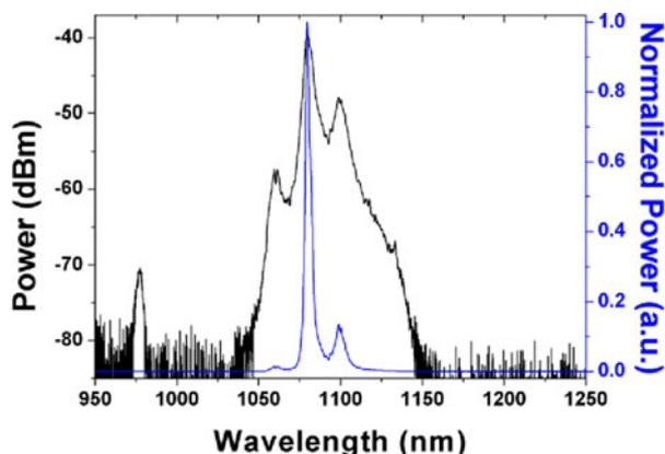
Fig. 3. The output spectrum for the amplified laser with a power of 5010 W.
