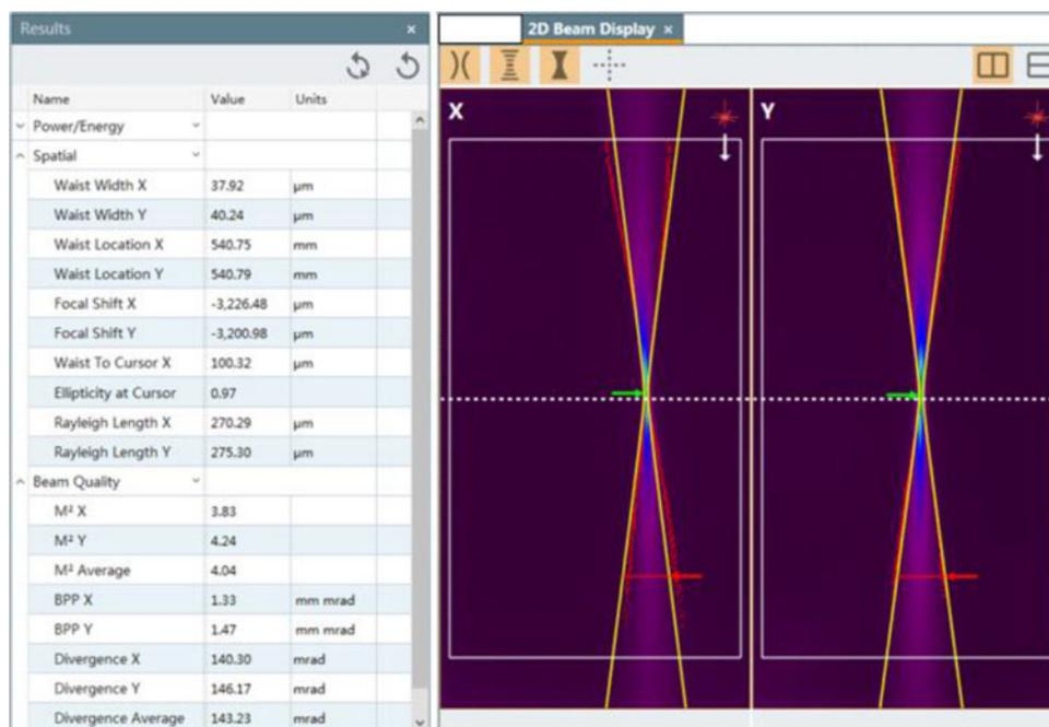
Fig. 8. The beam quality factor ( $M^2$ ) of the laser beam with 8050 W laser power.
