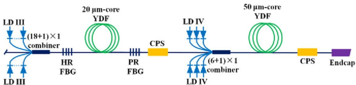
Fig. 5. Schematic configuration of the 8 kW high-brightness CW monolithic fiber laser.
