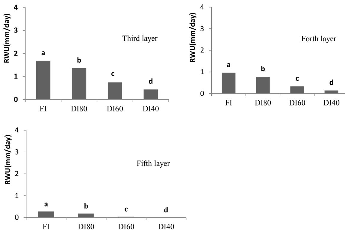
**Figure 2.** The averages of root water uptakes (ARWUs) in each layer of the soil in different treatments
