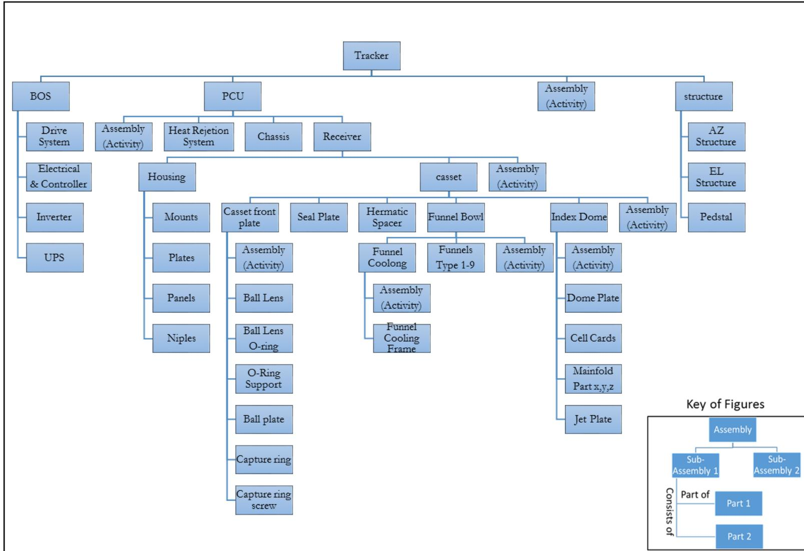
Figure 28: REhnu Second Generation CPV System Bill of Materials Diagram
