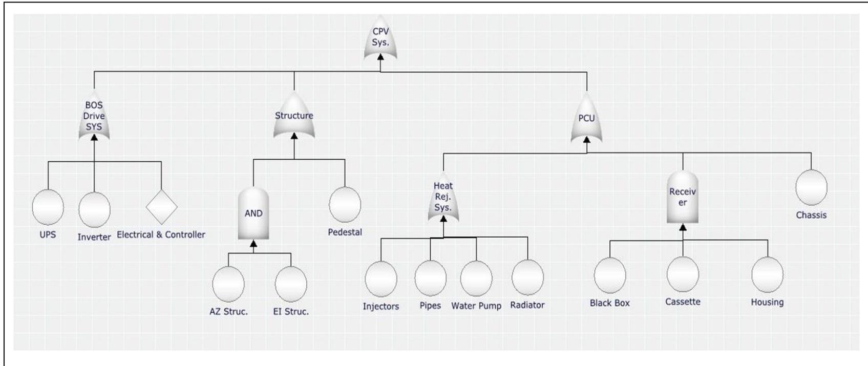
DARM's RDA FTA Analysis for the REhnu CPV System Using BlockSim /RENO
