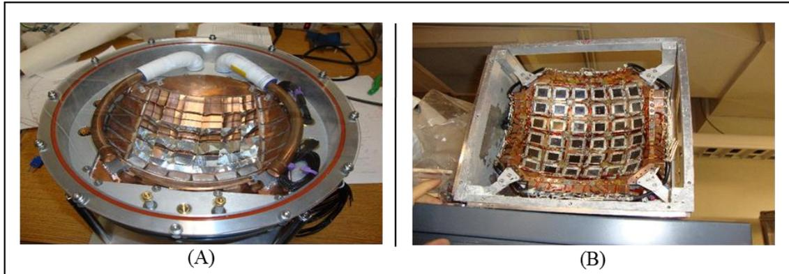
Figure 4: CPV Receiver Showing (A) Inside the Housing and (B) With the Solar Cells
