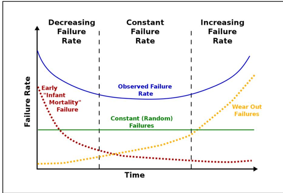
Figure 10: Failure Rate Bathtub Curve
