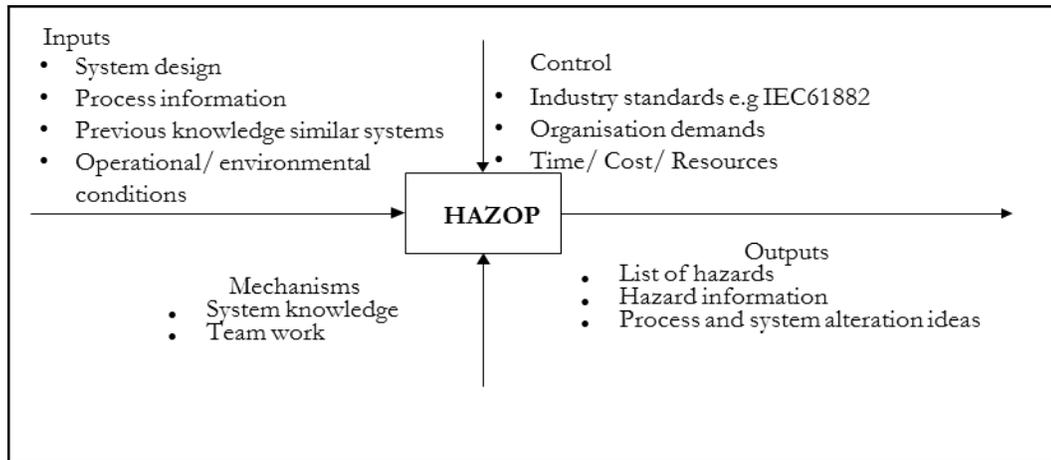
Figure 13: SADT Applied to HAZard and Operability Reliability Method
