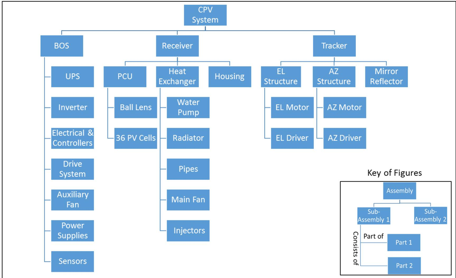
Figure 29: CPV System Functional Hierarchical Diagram
