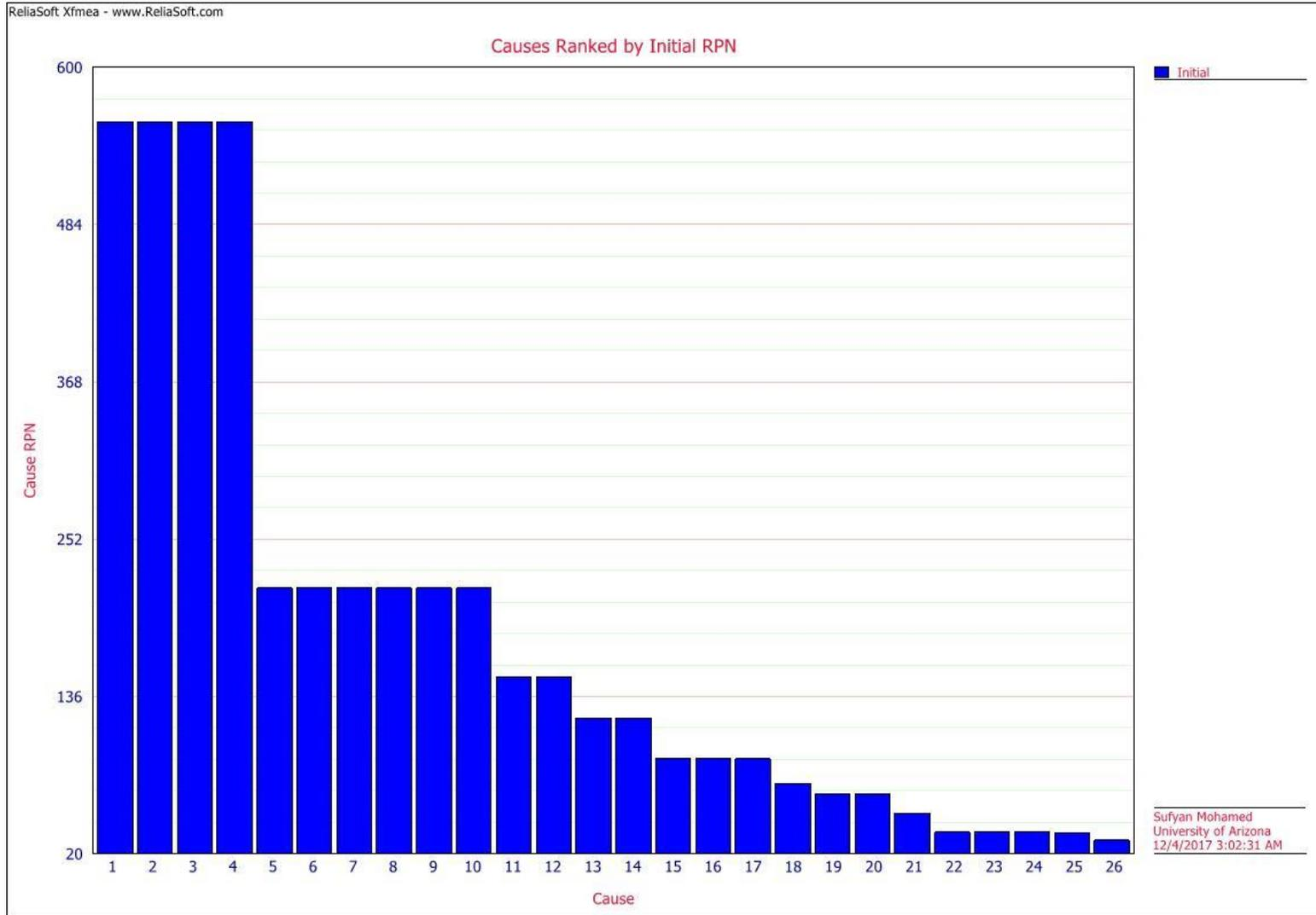
CPV system RPN diagram using FMEA
