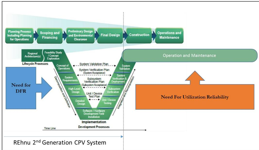
Figure 9: Design For Reliability and Utilization Reliability in System Life
