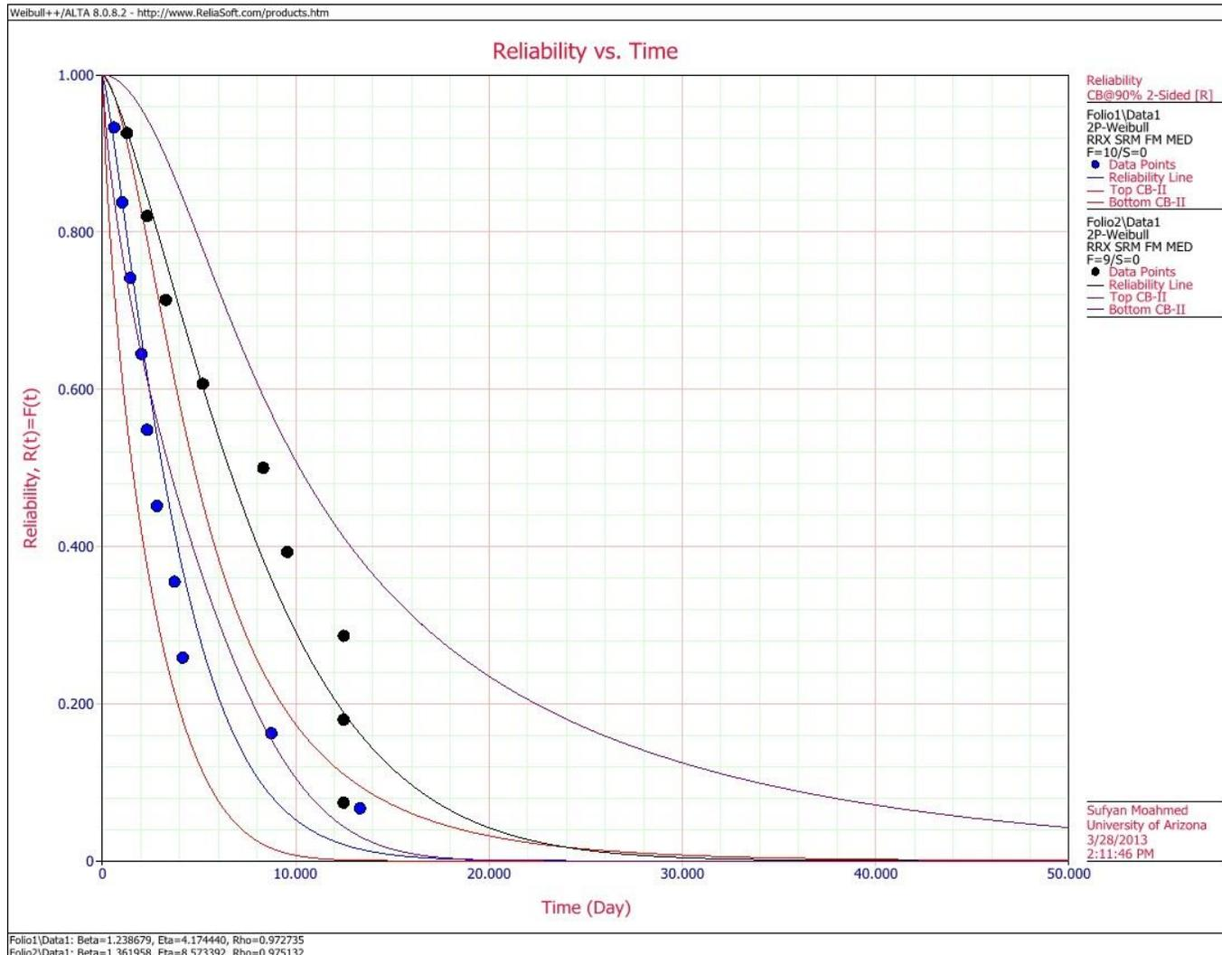
Reliability Function of the CPV System Using BlockSim
