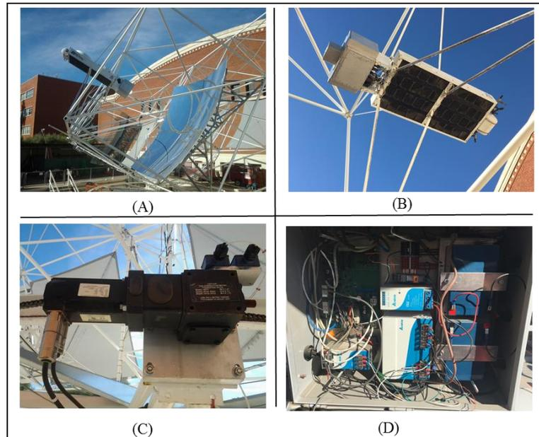
Figure 27: CPV Subsystems. A) Receiver, Tracker, and Reflector, B) Heat Exchanger, C) Motor, D) BOS
