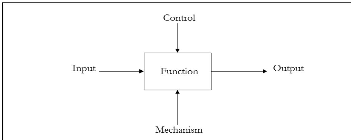
Figure 11: Structured Analysis and Design Technique (SADT) Model
