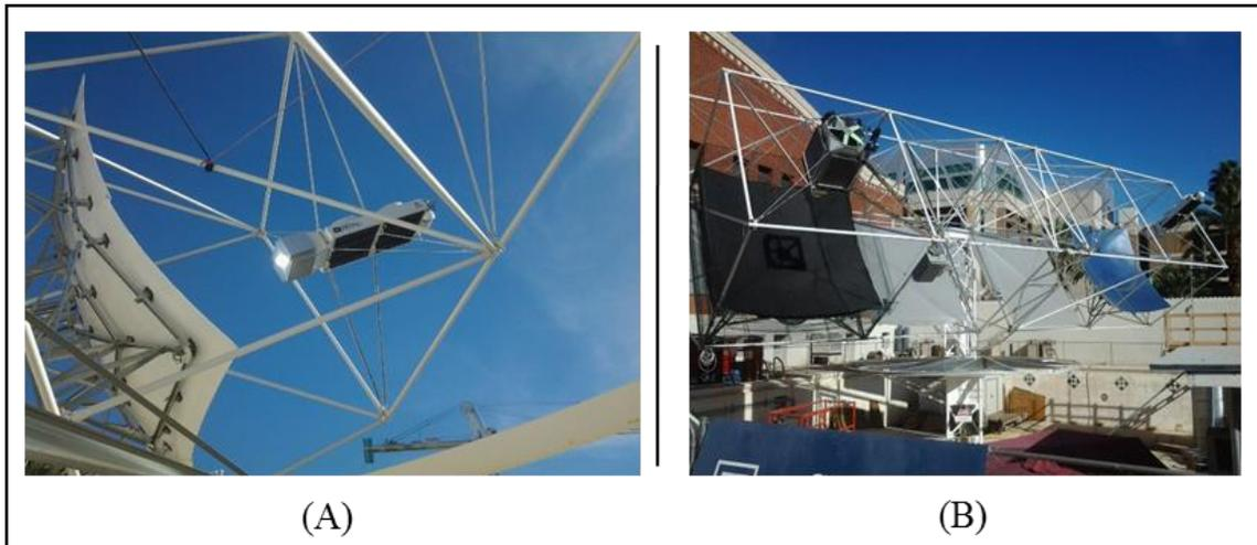
Figure 8: CPV Mechanical Subsystem Showing (A) Chassis, and (B) Tracker
