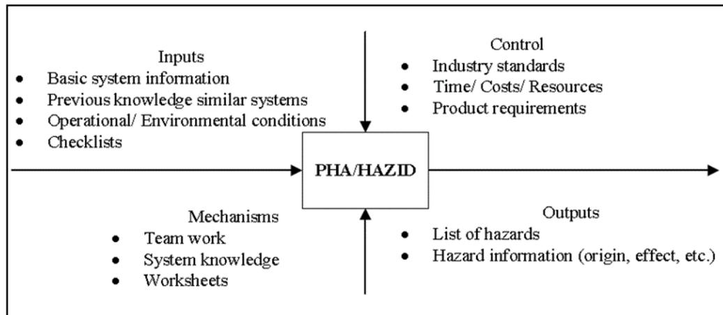
Figure 12: SADT Applied to Preliminary Hazard Analysis Reliability Method
