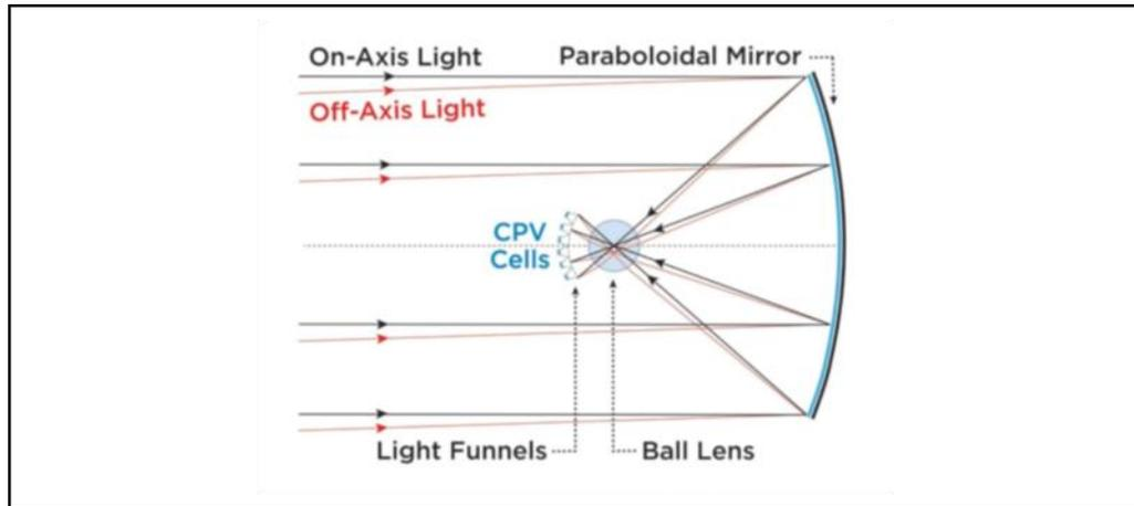
Figure 2: REhnu Second Generation CPV Mechanics and Operating Principle
