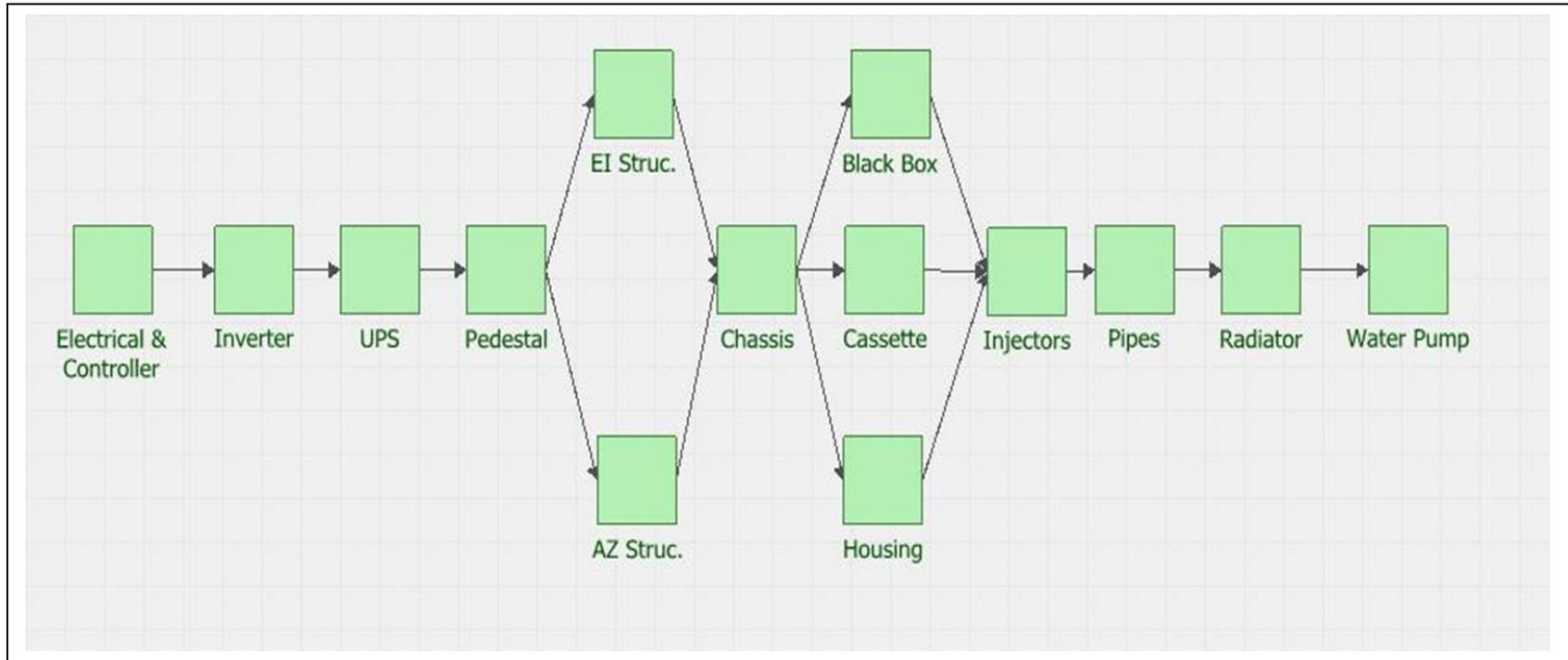
DARM's RDA RBD Analysis for the REhnu CPV System Using BlockSim /RENO
