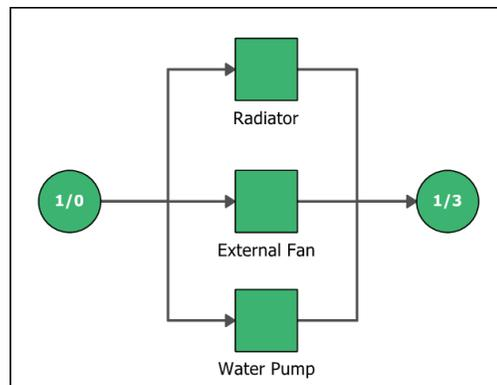
Figure 30: RBD of CPV Heat Exchange Subsystem
