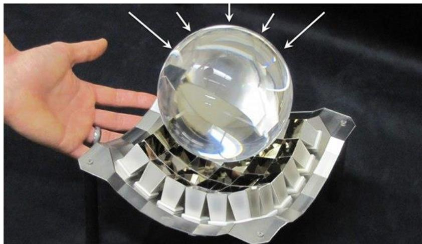
Figure 3: REhnu Second Generation CPV Ball Lens
