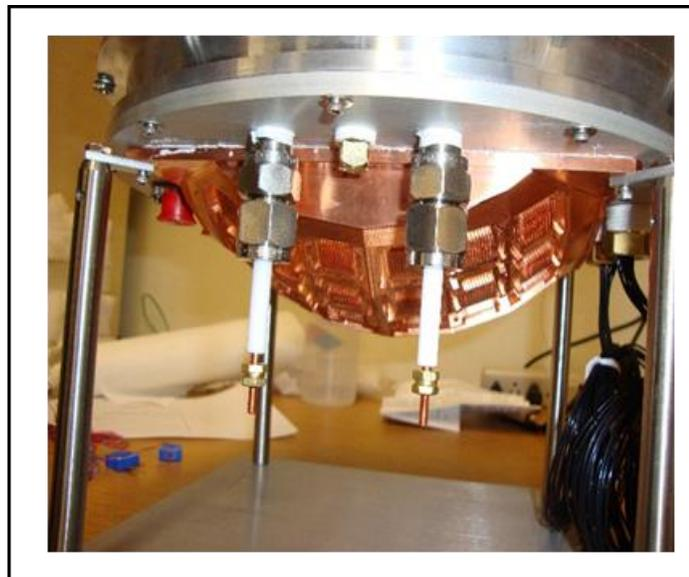
Figure 5: CPV Funnel Bowl Cooling Frame
