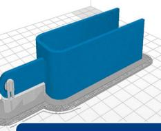
After customizing the device, the file can be downloaded in the standardized ".stl" format. With the download will come recommended instructions for build material, density, and orientation.
