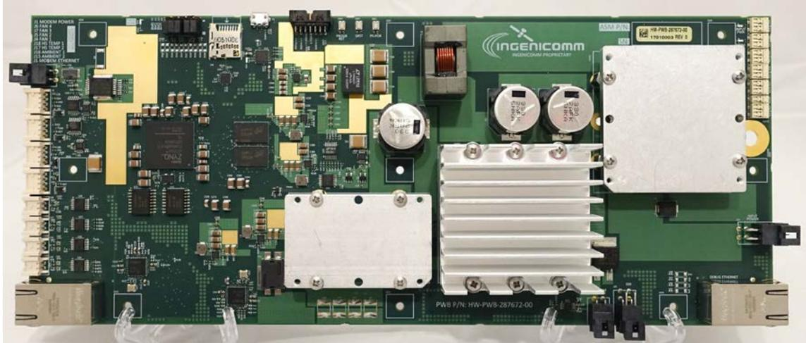
*Figure 3: Thermal Controller*
