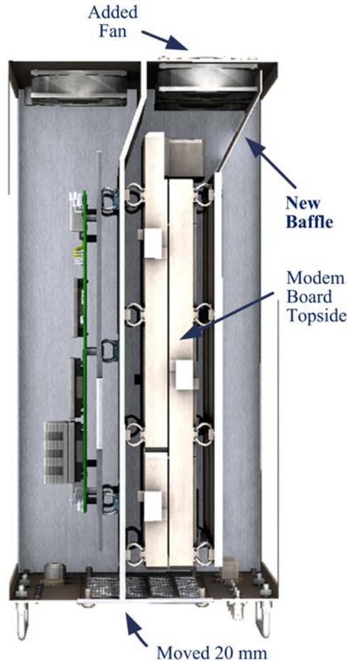
*Figure 4: Internal Airflow Channeling*
