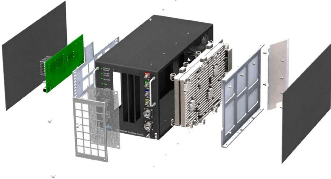
*Figure 1: Airborne Modem – Exploded View*
