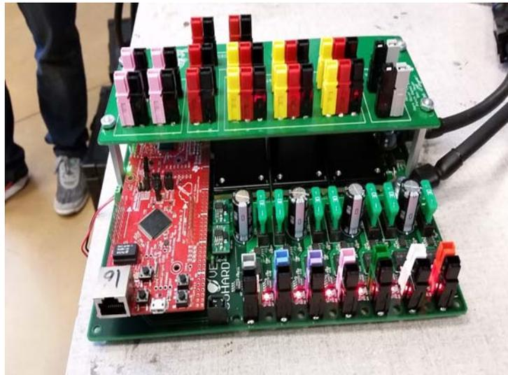
Figure 5: The Power Board with Its Seven Motor Buses and Four Specialized Buses
