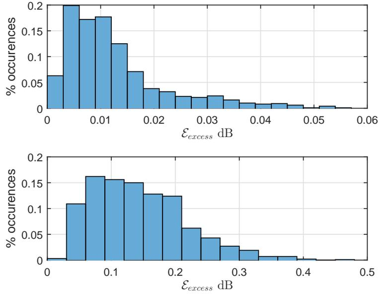
Figure 4: Increase of MSE with  $E_b/N_0 = 10$  dB for 1000 pairs of measured channel impulse responses from Cairns Army Airfield, Ft. Rucker, Alabama: (top) sparse MMSE equalizer with 25% active taps; (bottom) sparse MMSE equalizer with 10% active taps.
