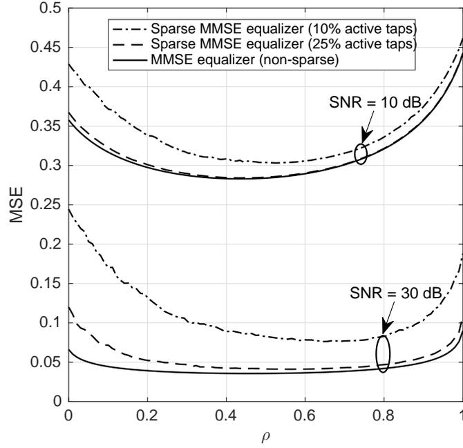
Figure 1: Plot of MSE vs power allocation parameter for GTR-STBC with both sparse and non-sparse MMSE equalizers. A pair of measured channel impulse responses from Cairns Army Airfield, Ft. Rucker, Alabama were used.
