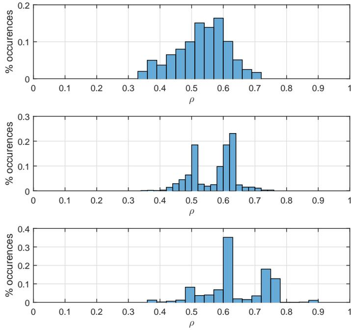
Figure 7: Optimum power allocations in the mean-squared error sense with  $E_b/N_0 = 16$  dB for 1000 pairs of measured channel impulse responses from Cairns Army Airfield, Ft. Rucker, Alabama: (top) non-sparse MMSE equalizer; (middle) sparse MMSE equalizer with 25% active taps; (bottom) sparse MMSE equalizer with 10% active taps.
