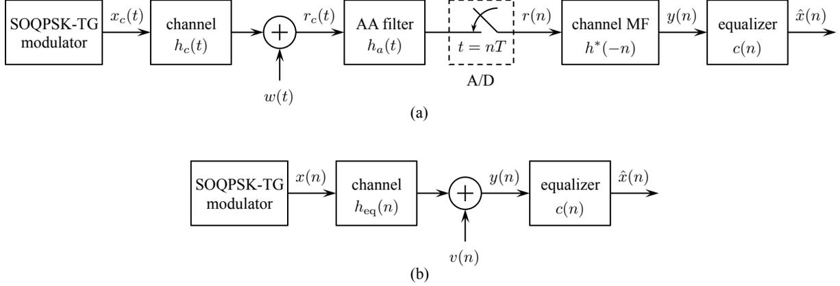
Figure 2: A block diagram of the system that applies an MMSE equalizer to samples of a received SOQPSK-TG signal: (a) the system showing the continuous-time signals, the anti-aliasing filter, and A/D converter; (b) the equivalent discrete-time system.
