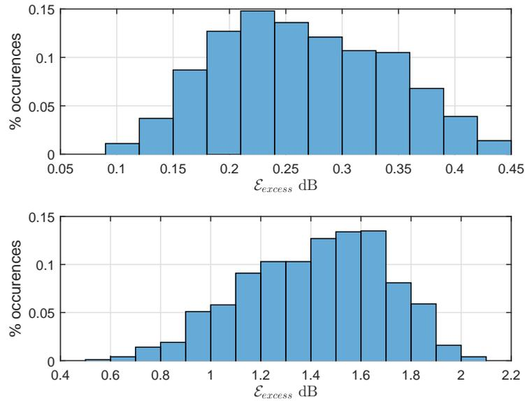
Figure 5: Increase of MSE with  $E_b/N_0 = 16$  dB for 1000 pairs of measured channel impulse responses from Cairns Army Airfield, Ft. Rucker, Alabama: (top) sparse MMSE equalizer with 25% active taps; (bottom) sparse MMSE equalizer with 10% active taps.
