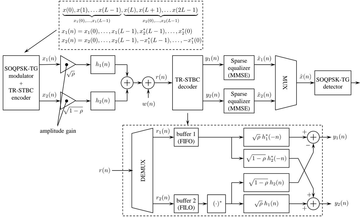
Figure 3: A block diagram of the TR-STBC system based on sparse equalizer and unequal power allocation using  $0 \leq \rho \leq 1$ .
