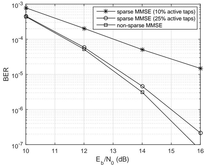
Figure 8: Comparison of average simulated BER for 1000 randomly selected channels from 39300 channel impulse responses measured at Cairns Army Airfield, Ft. Rucker, Alabama.
