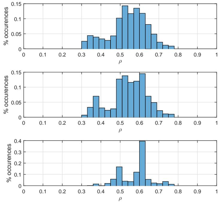
Figure 6: Optimum power allocations in the mean-squared error sense with  $E_b/N_0 = 10$  dB for 1000 pairs of measured channel impulse responses from Cairns Army Airfield, Ft. Rucker, Alabama: (top) non-sparse MMSE equalizer; (middle) sparse MMSE equalizer with 25% active taps; (bottom) sparse MMSE equalizer with 10% active taps.
