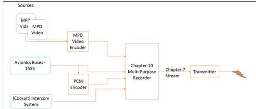
**Figure 2. Apache Instrumentation Scheme**
