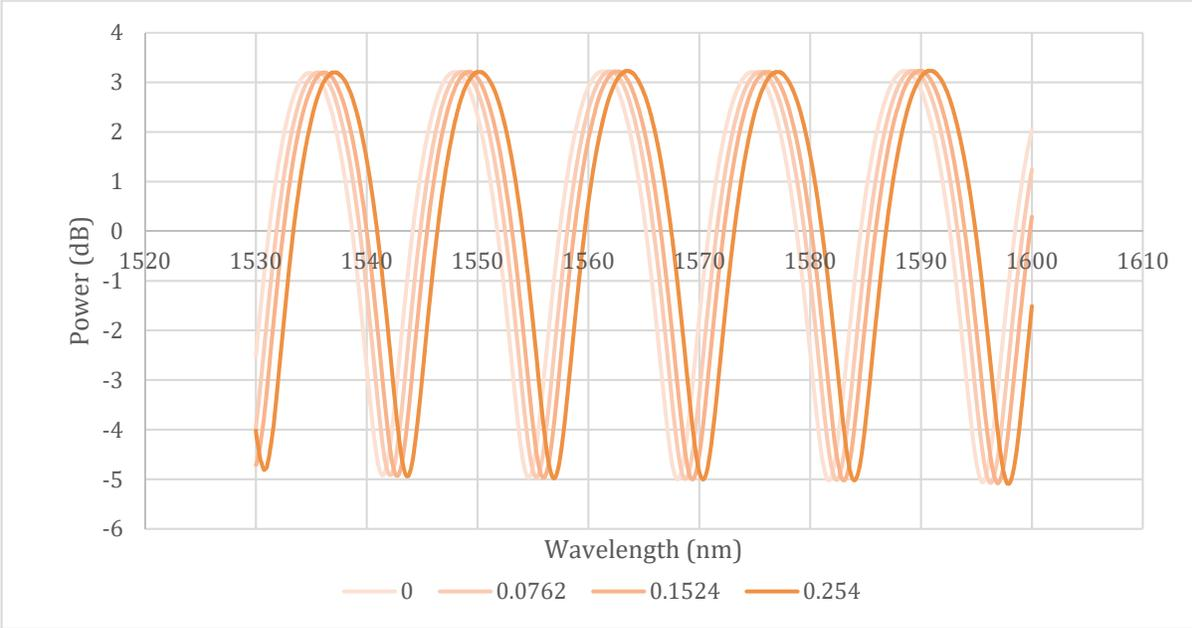
Figure 6 FPI Strain Testing Output Waveforms
