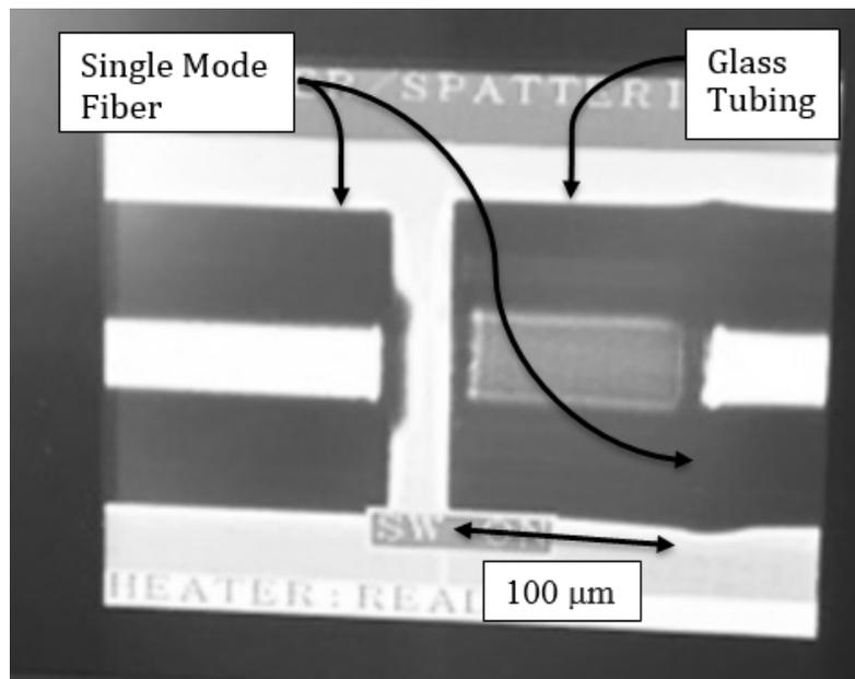
Figure 2 Fusing Single Mode Fiber with Glass Tubing
