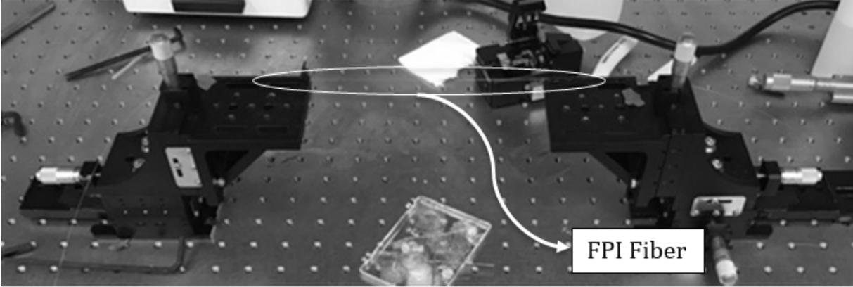
Figure 5 FPI Fixed to Moveable Plates
