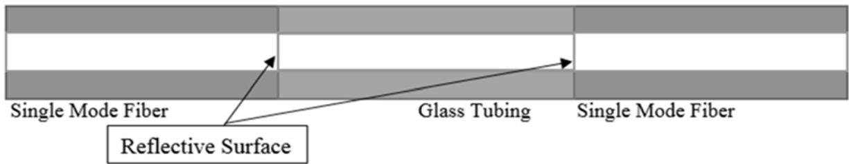
Figure 3 Fabry-Perot Interferometer
