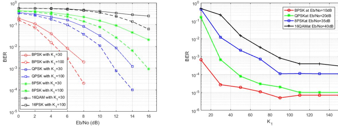
Figure 6: Impact of  $K_1$  on system Performance for Figure 7: Changes of BER versus  $K_1$  with  $K_2=30$ , SPACE08 Channel with  $K_2=40$  and  $K_3=40$ .  $K_3=30$  for SPACE08 Channel when  $E_b/N_0$  is fixed.
