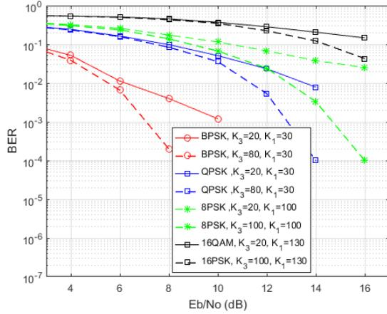
Figure 14: Impact of  $K_3$  on system Performance for SPACE08 Channel with  $K_2=50$ .
