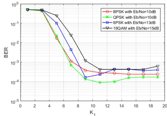
Figure 5: Changes of BER versus  $K_1$  with  $K_2=4$ ,  $K_3=3$  for Proakis Channel A when  $E_b/N_0$  is fixed.
