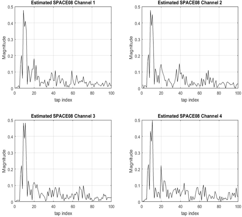
Figure 1: Tap Structure of the Magnitude of the Estimated SPACE08 Channel.
