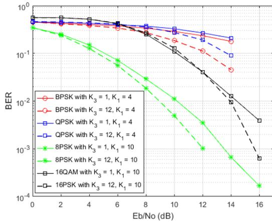
Figure 12: Impact of  $K_3$  on system Performance for Proakis Channel A with  $K_2=4$ .
