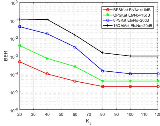
Figure 15: Changes of BER versus  $K_3$  with  $K_1=40$ ,  $K_3=40$  for SPACE08 Channel when  $E_b/N_0$  is fixed.
