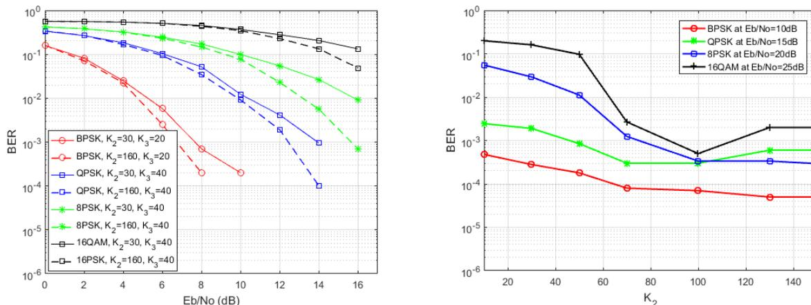
Figure 10: Impact of  $K_2$  on system Performance for SPACE08 Channel with  $K_1=100$ . Figure 11: Changes of BER versus  $K_2$  with  $K_1=50, K_3=30$  for SPACE08 Channel when  $E_b/N_0$  is fixed.
