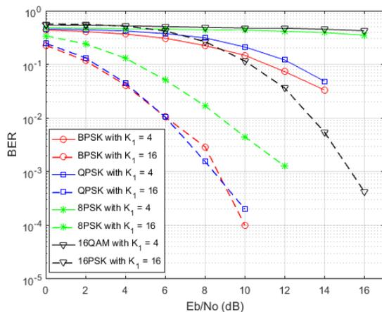
Figure 4: Impact of  $K_1$  on system Performance for Proakis Channel A with  $K_2=4$  and  $K_3=3$ .
